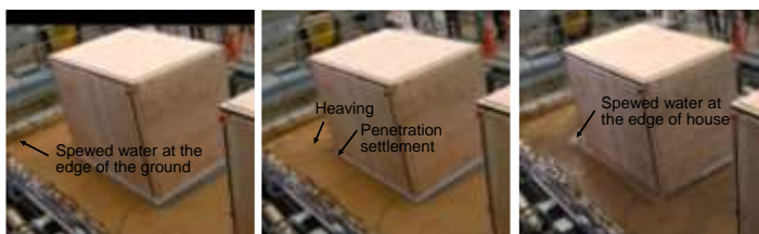
(a) Spewed water at the edge of the ground at 26 sec. (b) Penetration settlement at 34 sec. (c) Spewed water at the edge of house around 70 sec.
