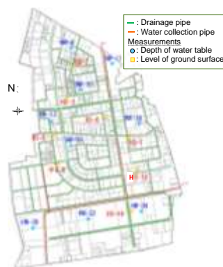
Fig. 28 Layout of drainage pipes in Hirai-tohbu in Kashima City (Yasuda et al., 2020)
