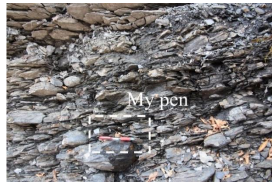
Fig. 15 Fractured rock of Ohya landslide site
