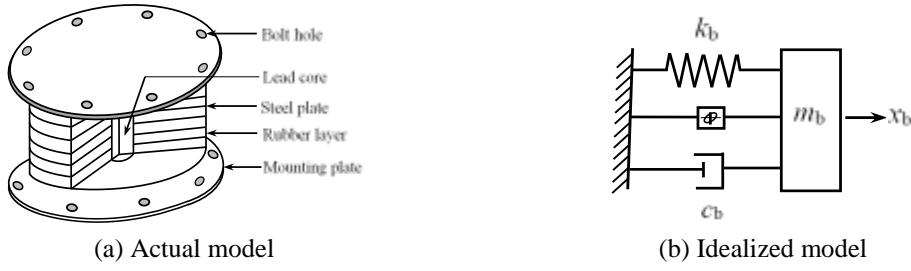
Fig. 2 Schematic representation of lead rubber bearing (LRB)
