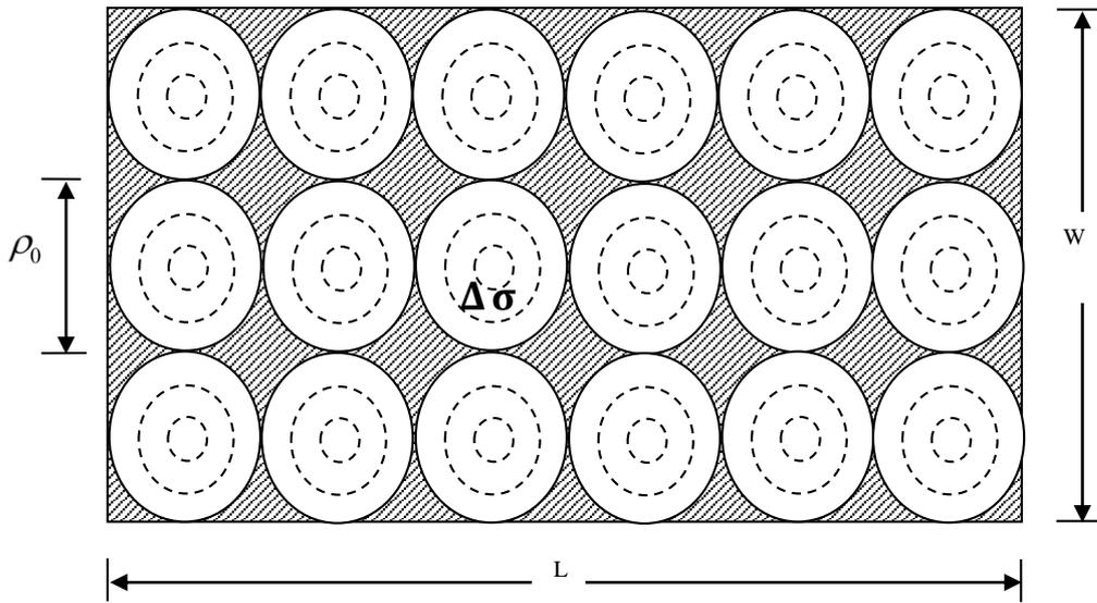
Fig. 3 Schematic view of specific barrier model (Papageorgiou and Aki [24])
