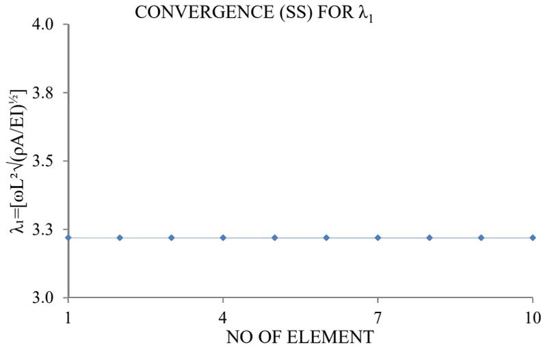
Fig. 4 Convergence study for natural frequency for 1<sup>st</sup> mode of a simply supported (S - S) beam
