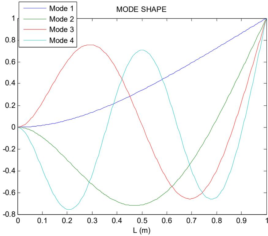
Fig. 8 Mode shape of clamped-free (C - F) beam
