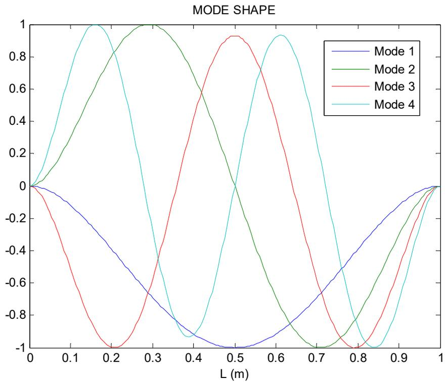
Fig. 6 Mode shape of clamped-clamped (C - C) beam
