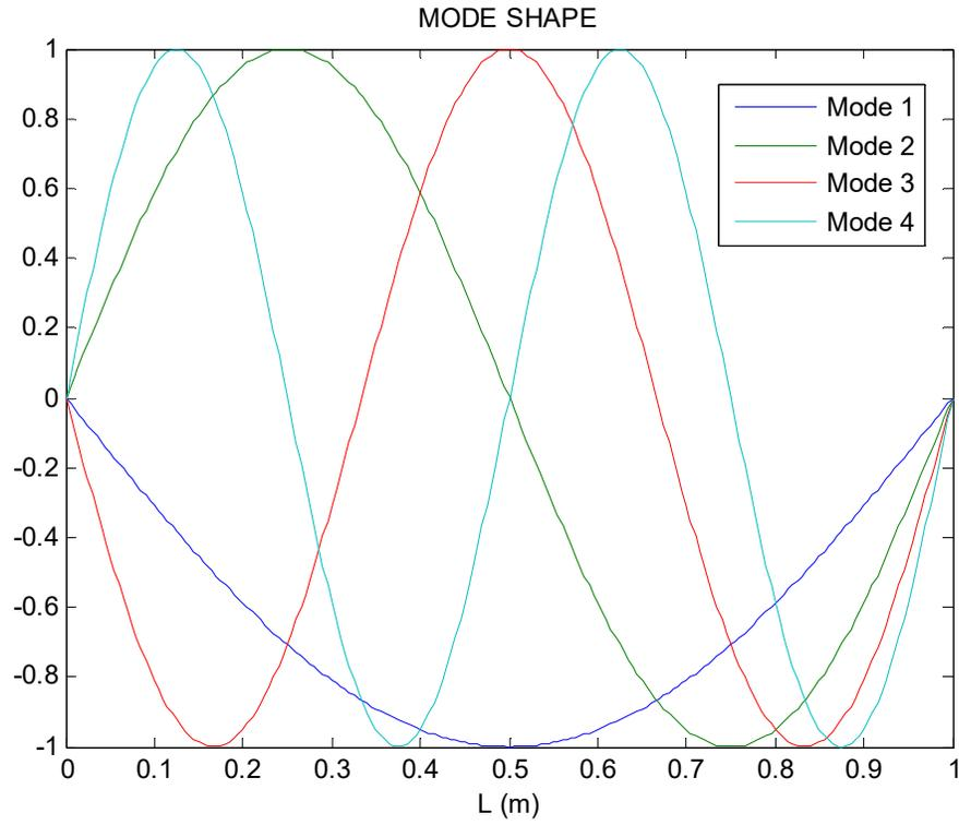
Fig. 7 Mode shape of S - S beam
