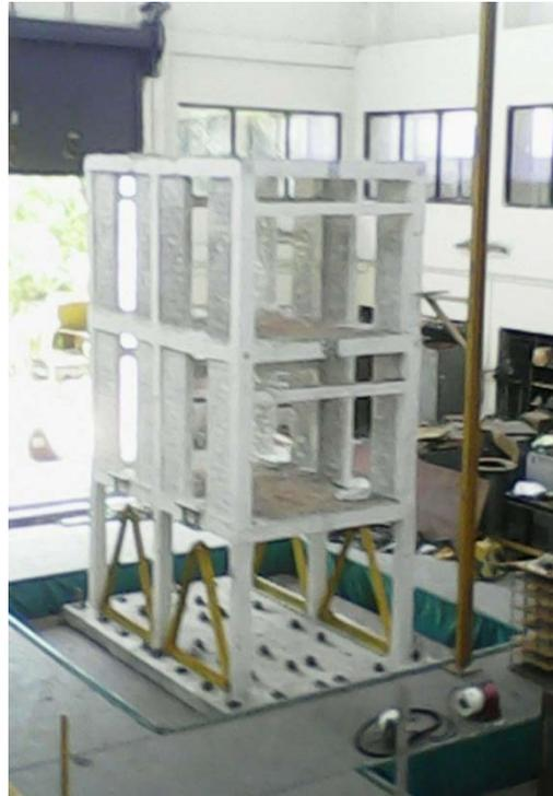
Fig. 14 XPD connections in ground story of RC building
