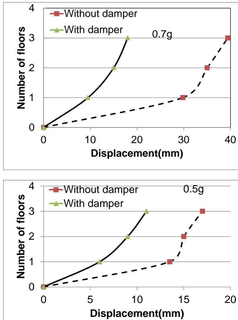
Fig. 15 Comparison of relative displacement of building for different cases of earthquake with and without damper
