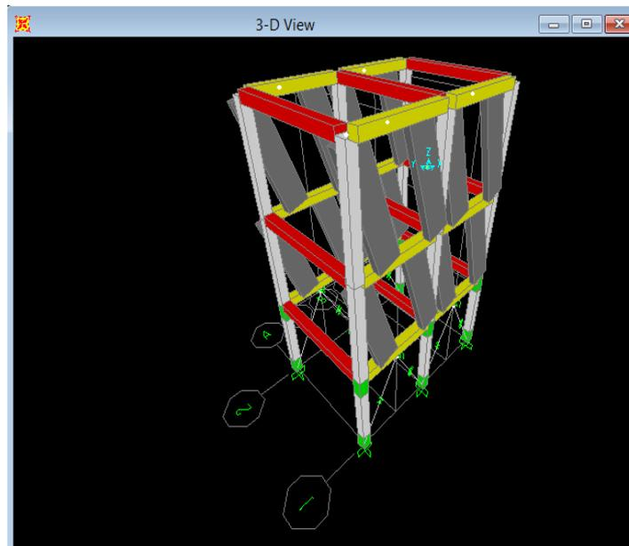
Fig. 12 3D view of original building in SAP2000 after retrofitting
