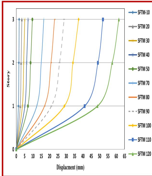
Fig. 5 Peak storey displacement for various seismic inputs
