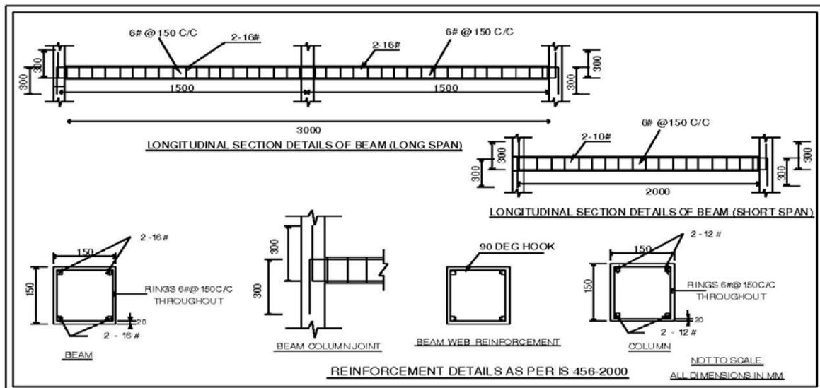
Fig. 2 Reinforcement details of beam and column and dimensions
