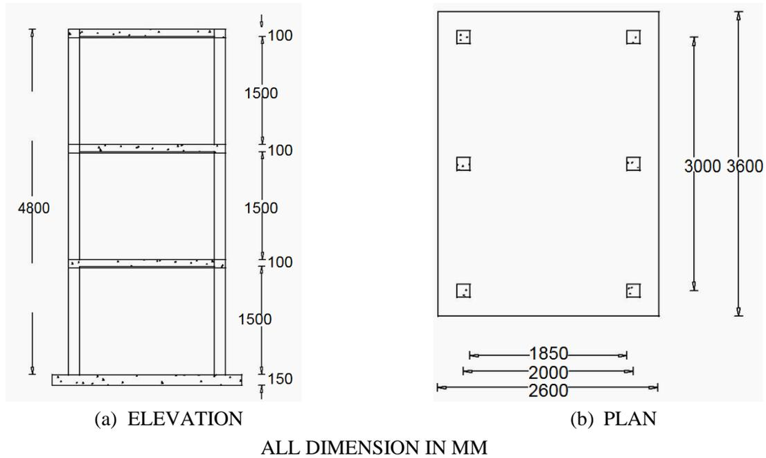
Fig. 3 Details of RC frame building
