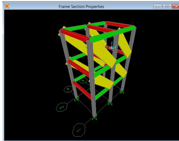
Fig. 11 3D view of original building in SAP2000 before retrofitting
