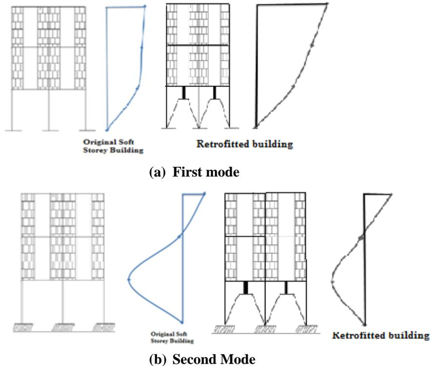
Fig. 10 First mode and second mode shapes of RC building with X-shaped metallic damper
