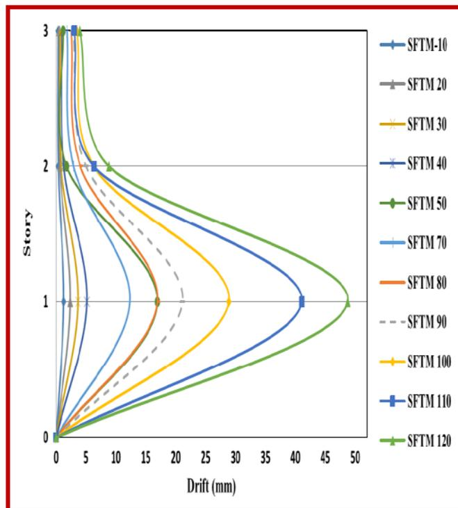
Fig. 6 Peak storey drift for various seismic inputs
