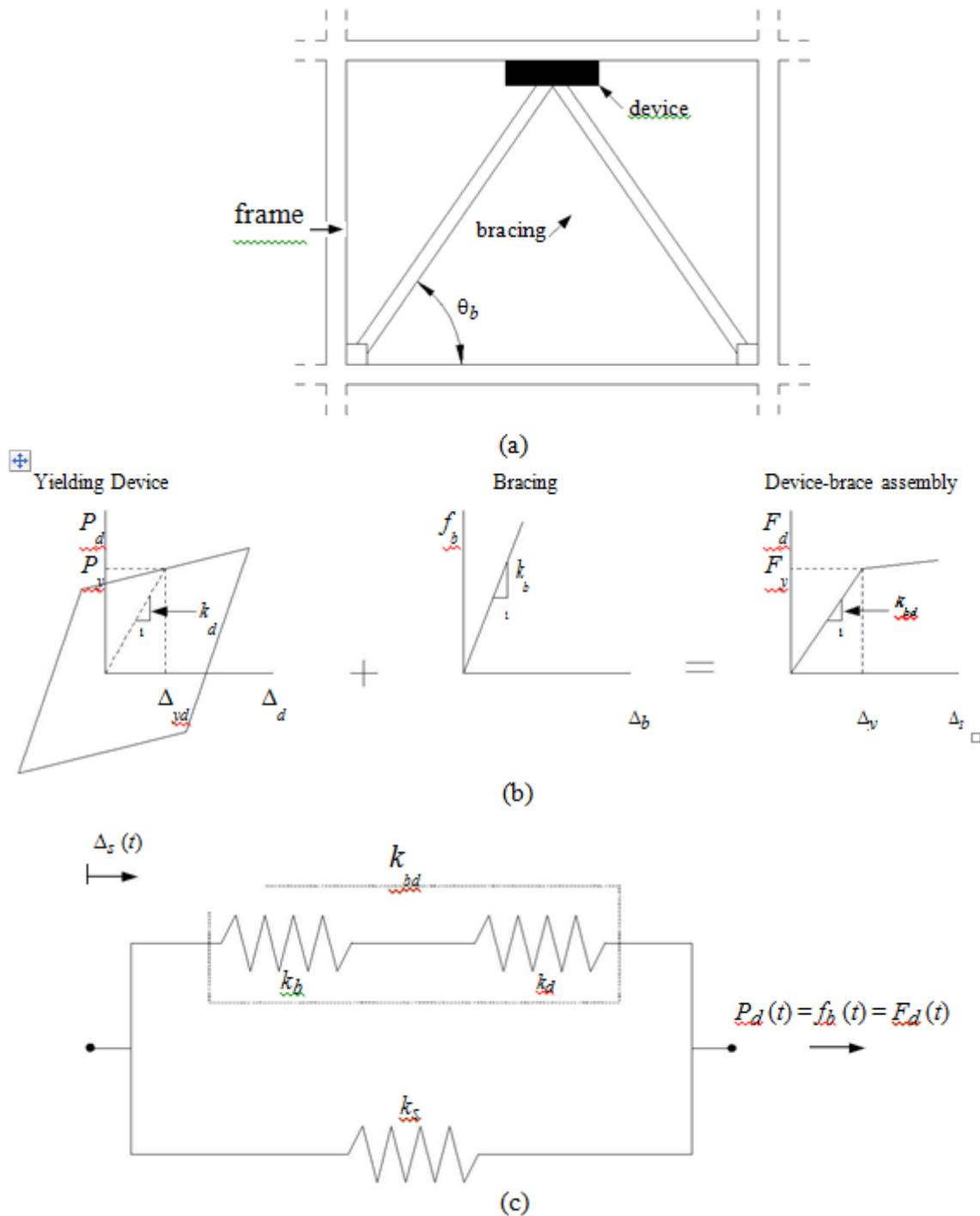
Fig. 7 Yielding metallic damper, (a) typical configuration, (b) yielding metallic device, bracing and yielding element parameters, (c) stiffness properties of device-bracing assembly
