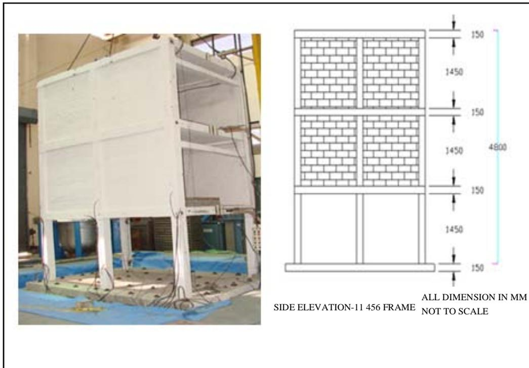
Fig. 1 View of Reinforced concrete building and dimensions
