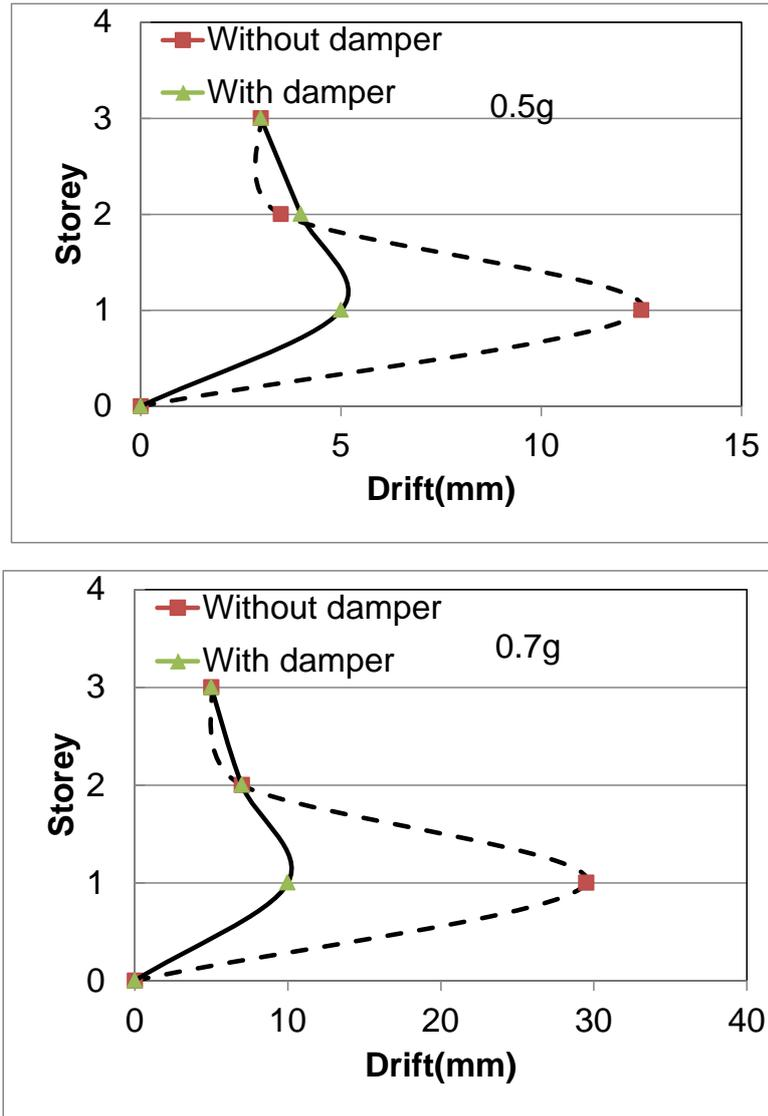
Fig. 16 Comparison of storey drift of building for different cases of earthquake with and without damper
