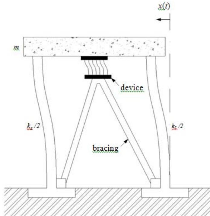
Fig. 8 Idealized building structure with supplemental yielding metallic element
