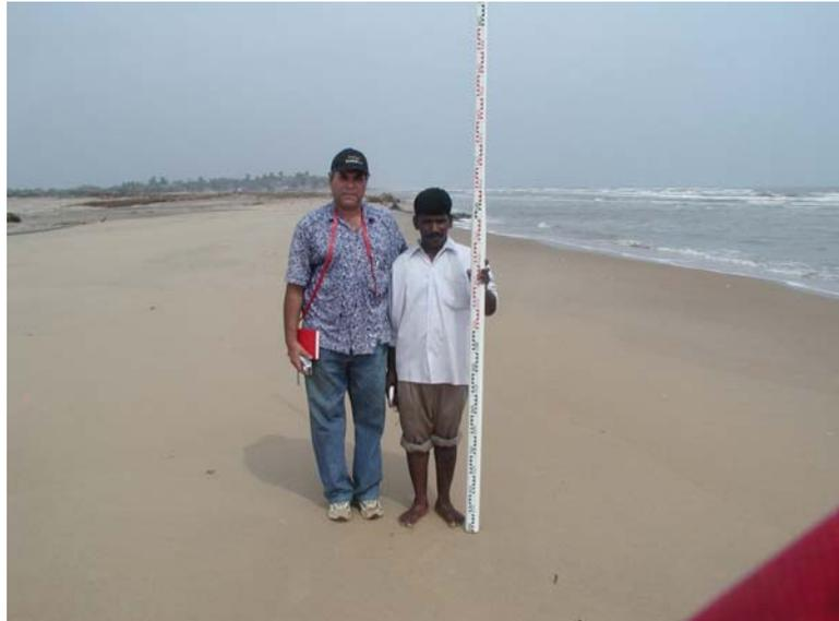
Fig. 4 Photograph of stadia rod near beach endpoint of profile NAGA01 (10 m position) with swash zone at the right (stadia rod was held at mid-swash, i.e. mean water level, to establish timed tide level during survey)
