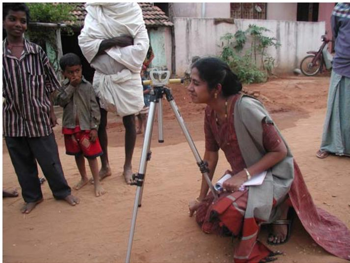
Fig. 3 Photograph of level and tripod setup on profile PERI01 (170 m position) for shooting level line from tsunami high-water deposits to beach swash zones
