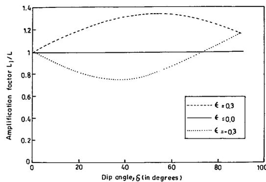
Fig. 4 Variation of the amplification factor  $L_I/L$  with the dip-angle for  $\gamma = C_{55}/C_{44} = 1$  and for three values of the anisotropy parameter  $\varepsilon = -C_{45}/C_{44}$ , namely,  $\varepsilon = 0, 0.3, -0.3$  ( $\varepsilon = 0$  corresponds to the isotropic half-space)
