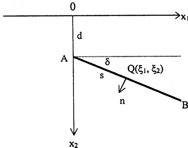
Fig. 1 Geometry of a long fault in a half-space (The fault is of infinite length in the strike ( $x_3$ )-direction.  $AB$  is the fault section by the  $x_1x_2$ -plane which is also the plane of elastic symmetry of the monoclinic elastic half-space  $x_2 \geq 0$ ,  $d$  is the depth of the upper edge  $A$  of the fault and  $\delta$  the dip angle.  $(s, \delta)$  denote the polar coordinates of any point  $Q(\xi_1, \xi_2)$  on the fault.)
