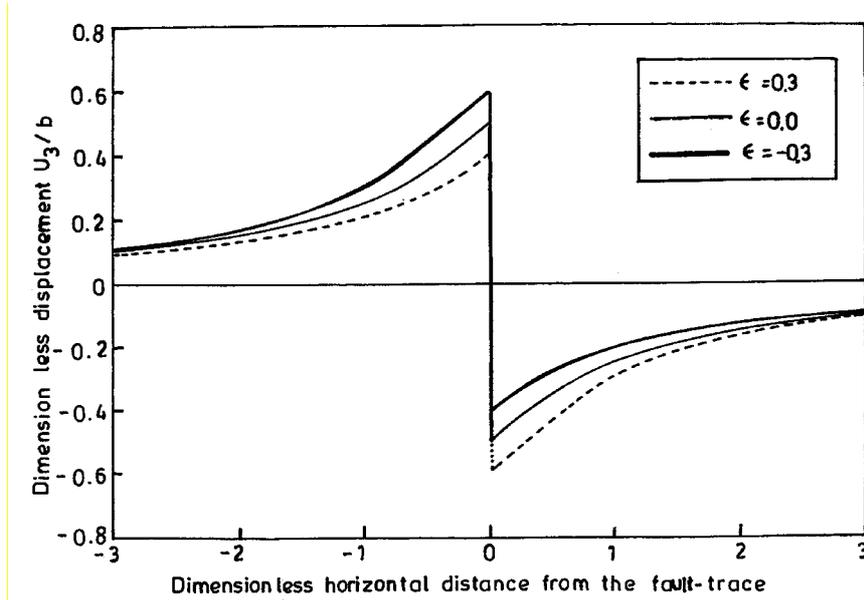
Fig. 5 Variation of the dimensionless along-strike surface displacement ( $u_3/b$ ) with the dimensionless horizontal distance ( $x_1/L$ ) from the upper edge of a surface-breaking vertical fault for  $\gamma=1$  and  $\varepsilon=0, +0.3, -0.3$
