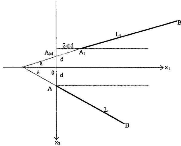
Fig. 2 Showing the source fault  $AB$  of width  $L$  and the image fault  $A_1B_1$  of width  $L_1$  for a monoclinic half-space  $x_2 \geq 0$  (The source fault makes an angle  $\delta$  with the horizontal, and the image fault makes an angle  $\delta_1$  with the horizontal in the opposite sense. The image fault in the case of a monoclinic half-space does not coincide with the mirror image of the source fault in the free boundary.)
