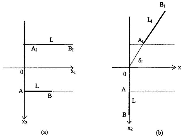
Fig. 3 Showing the image fault when the source fault is (a) parallel to the boundary, and (b) perpendicular to the boundary
