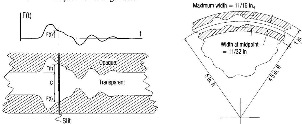
Fig. 3 Left: Transformation of input function to variable-width film trace, Right: Dimensions of the standard film disk record for the function generator (redrawn from Caughey et al. (1960))
