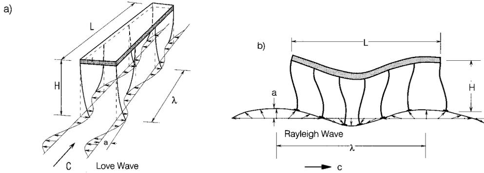
Fig. 11 (a) Deformation of columns in a two-degree-of-freedom system, during out-of-plane response, excited by Love waves, (b) Deformation of columns in a long structure during in-plane response and excited by Rayleigh waves
