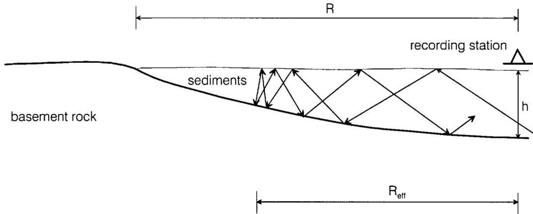
Fig. 5 Reflection of trapped waves from the edge of a sedimentary valley (*h* is the depth of sediments under the station, *R* is the distance to the reflecting rock, as it is seen on the earth’s surface, and *R<sub>eff</sub>* is the “effective” distance from the station to the region where the reflection actually occurs)
