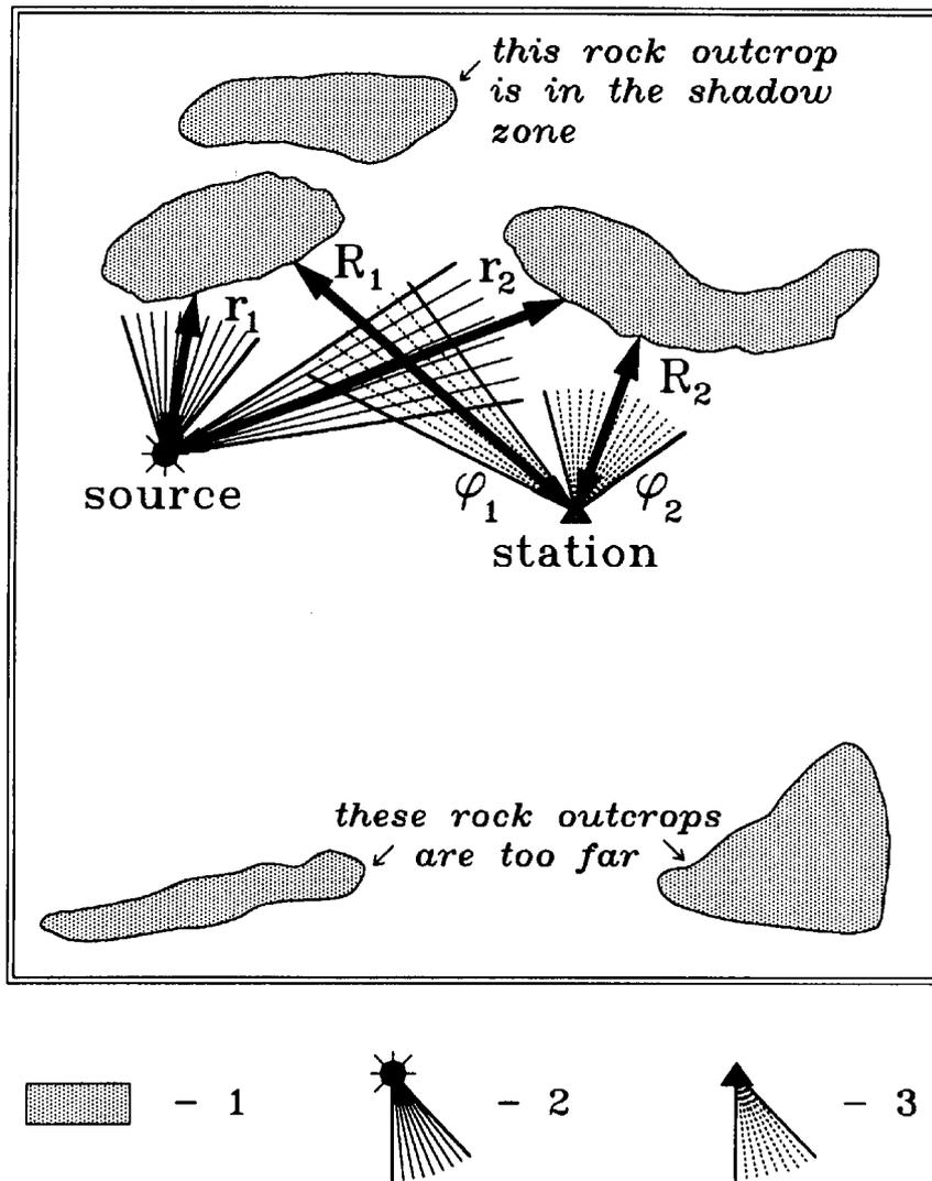
Fig. 4 A representation of  $R$  and  $\phi$  ("1" shows the basements rocks on the earth's surface; "2" is the angle, subtended at the source by the rocks from which reflection occurs; the solid lines represent the direct waves; "3" is the angle, subtended at the recording station by the surface of the rocks from which reflection occurs; the dashed lines represent the waves reflected by the rock towards the station)
