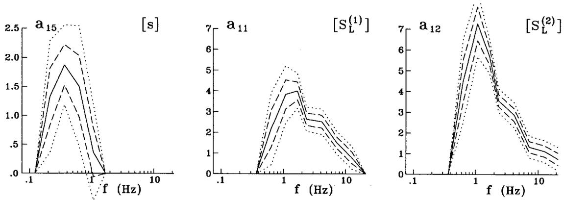
Fig. 8(b) The coefficients  $a_{15}(f)$ ,  $a_{11}(f)$  and  $a_{12}(f)$  in the model in Equation (13) plotted versus central frequency of the channel (solid lines) (the dashed lines indicate the “ $\sigma$ -intervals”, and the dotted lines indicate the 95% confidence intervals)
