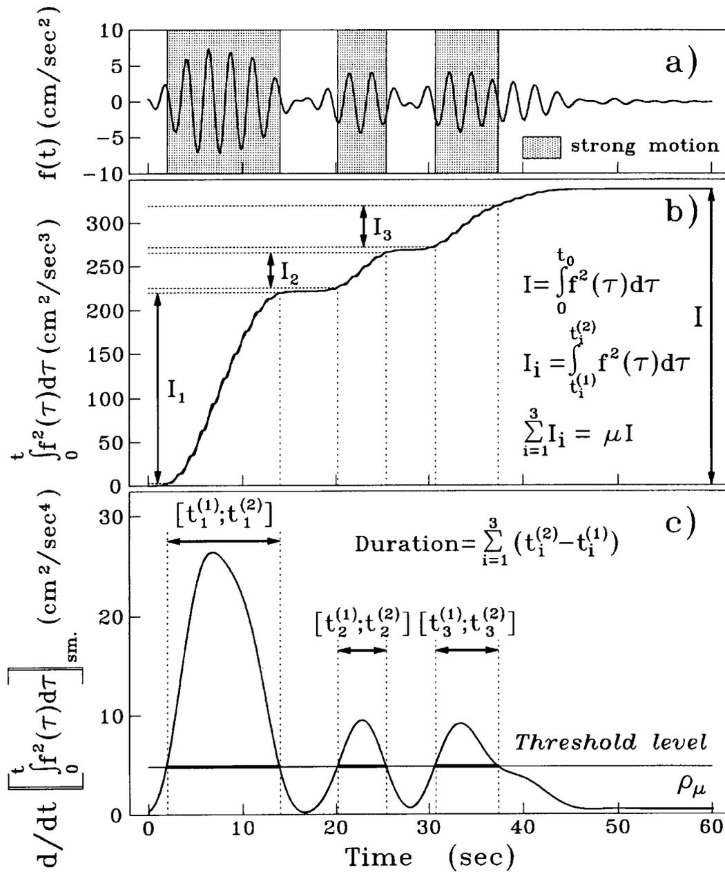
Fig. 1 The definition of duration for an acceleration component, (band-pass filtered, central frequency 0.37 Hz): a) time history  $f(t)$  (the strong motion intervals are shaded); b)  $\int_0^t f^2(\tau) d\tau$ ; c) the derivative of the integral of  $f^2(t)$  after smoothing and the threshold level  $\rho_\mu$  (the time intervals giving contribution to duration with  $\mu = 0.9$  are highlighted)
