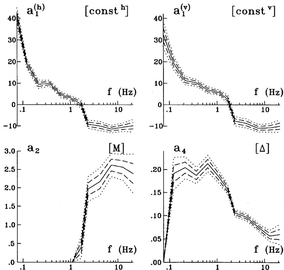
Fig. 8(a) The coefficients  $a_1(f)$ ,  $a_2(f)$  and  $a_4(f)$ , in the model in Equation (13) plotted versus central frequency of the channel (solid lines) (the dashed lines indicate the “ $\sigma$  - intervals”, and the dotted lines indicate the 95% confidence intervals)
