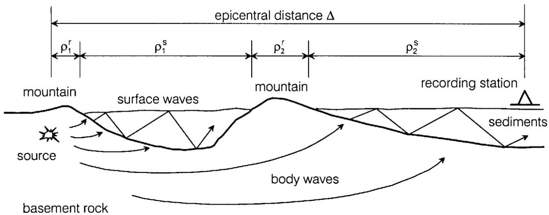
Fig. 2 The strong motion energy reaches the station in form of the surface waves and body wave
