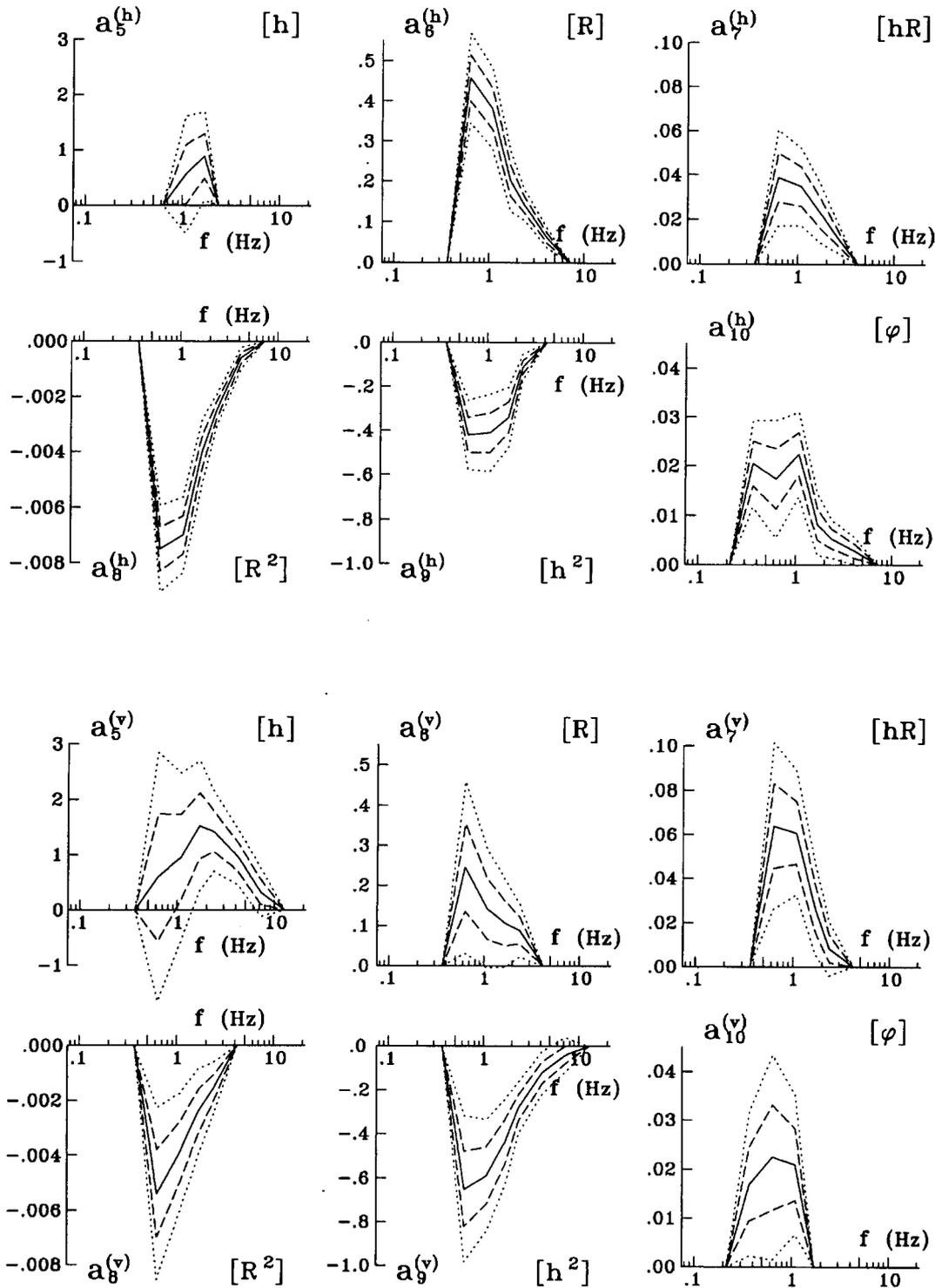
Fig. 6(b) Coefficients  $a_5$  through  $a_{10}$  in Equation (11), versus central frequency of the channels (solid lines) (the dashed lines indicate the “ $\sigma$ -intervals” and the dotted lines indicate the 95% confidence intervals)
