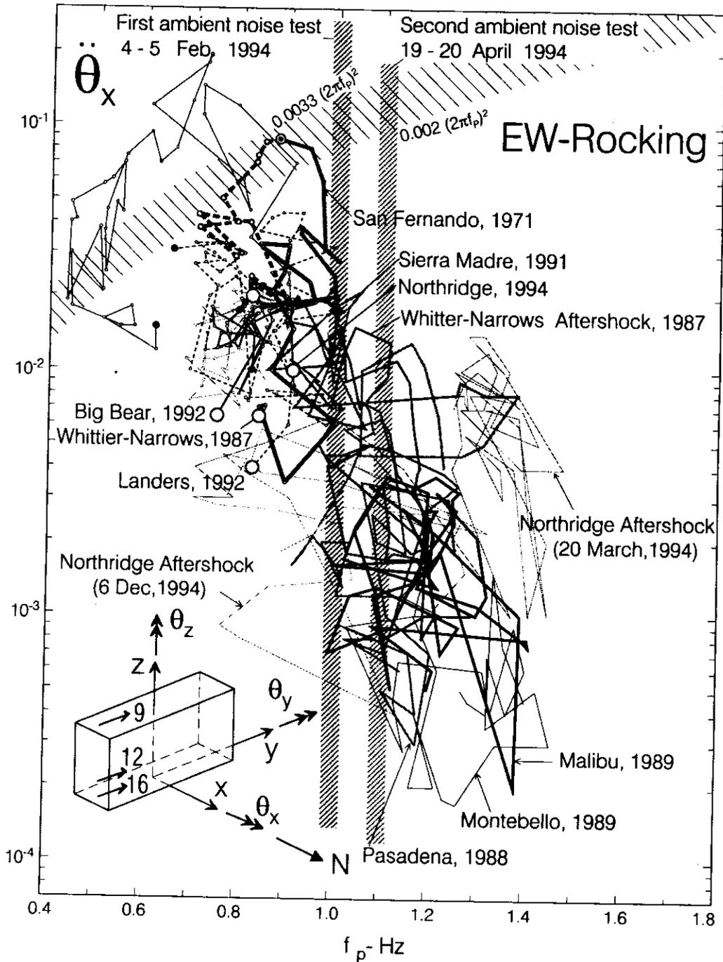
Fig. 15 Peak amplitudes of  $\ddot{\theta}_x$  (EW rocking acceleration) versus  $f_p$  (apparent frequency of the soil-foundation-structure system) during twelve earthquakes (see Fig. 2). (the gray vertical lines show the apparent EW frequencies of the system response as determined from Experiments I and II)
