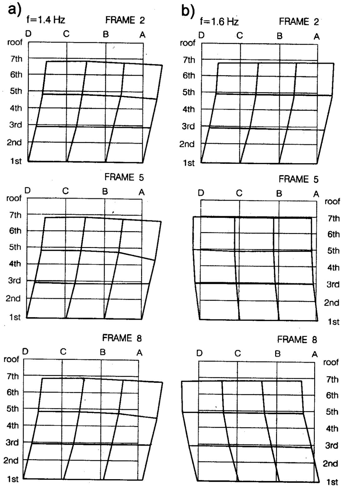
Fig. 14 Experiment II - in-plane displacements of transverse frames 2, 5 and 8: (a) at the frequency of the first transverse mode ( $f = 1.4$  Hz) and (b) at the frequency of the first torsional mode ( $f = 1.6$  Hz)
