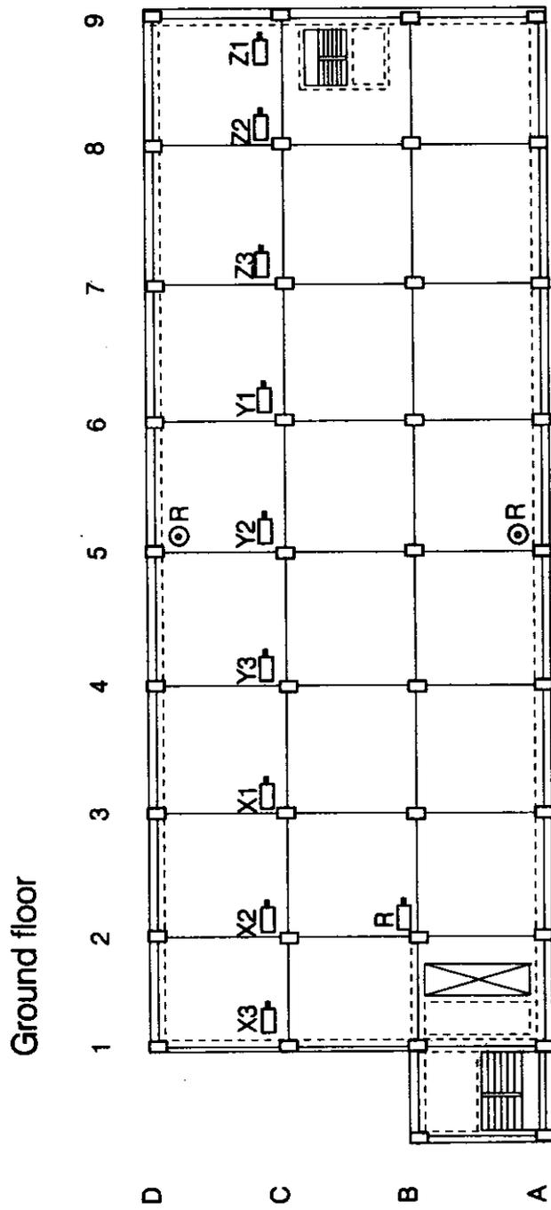
Fig. 9 Experiment II: position of instruments on the ground floor
