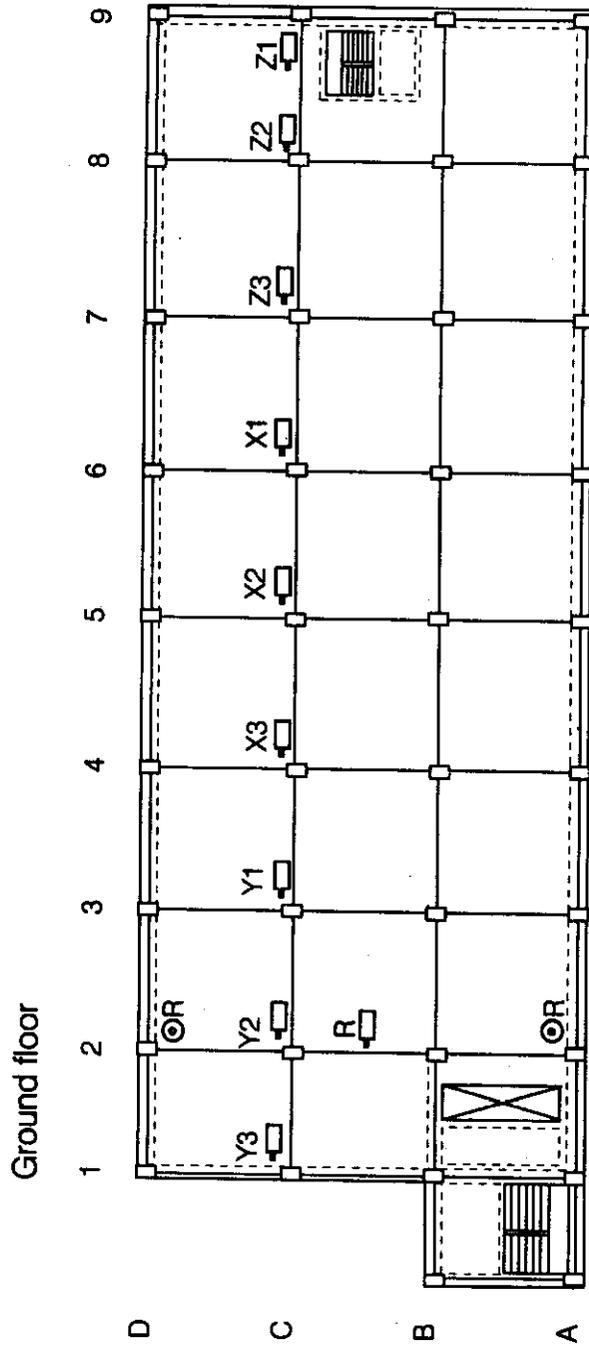
Fig. 6 Experiment I: position of instruments on the ground floor
