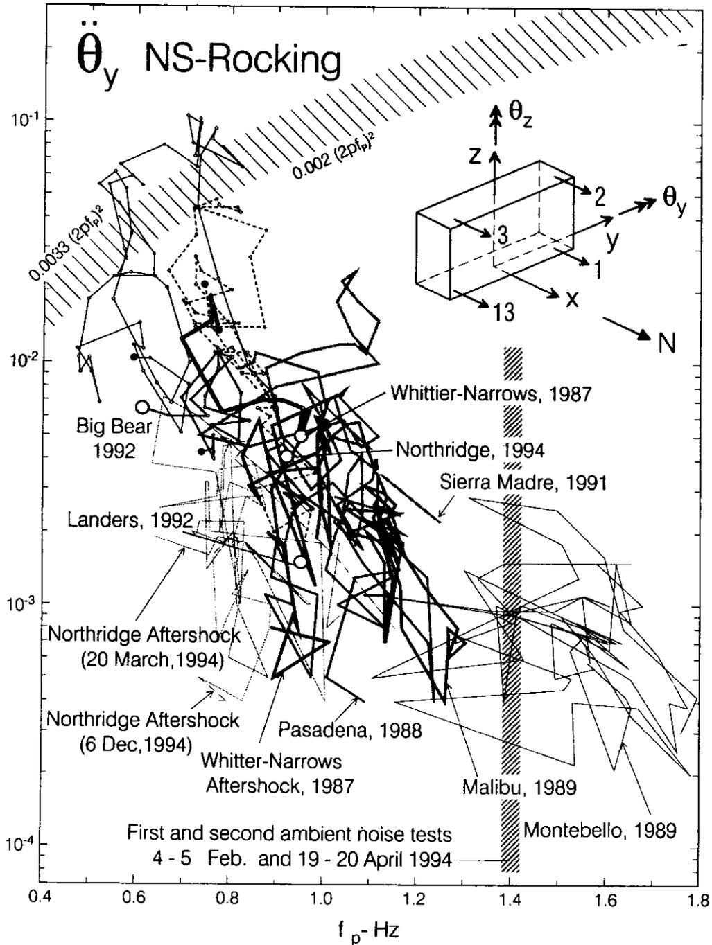
Fig. 16 Peak amplitudes of  $\ddot{\theta}_y$  (NS rocking acceleration) versus  $f_p$  (apparent frequency of the soil-foundation-structure system) during twelve earthquakes (see Fig. 2) (the gray vertical line shows the apparent EW frequency of the system response as determined from Experiments I and II)
