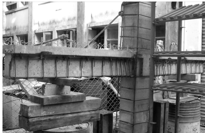
Fig. 12 Fabrication of reinforcement for retrofitted sub-assembly specimens
