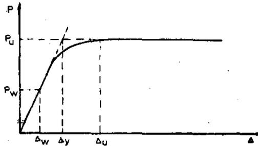
Fig. 1 Lateral load deflection curve
