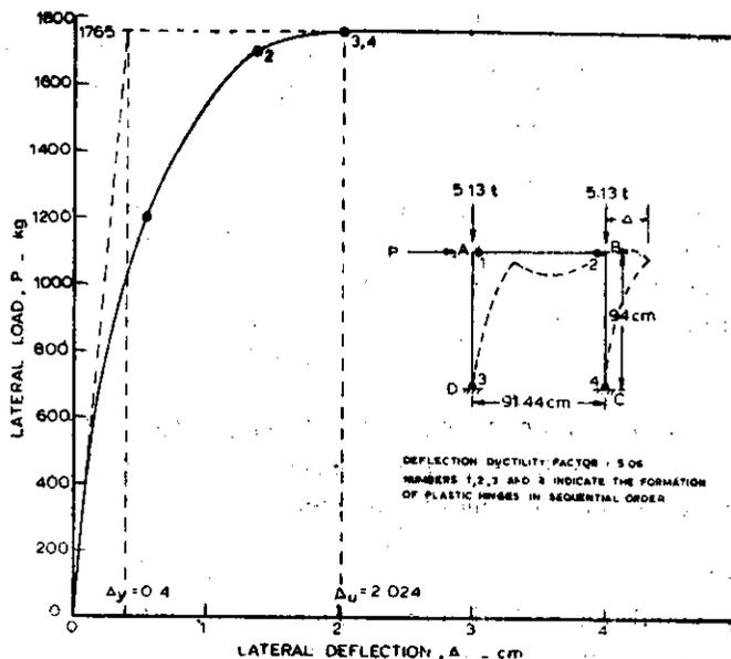
Fig. 3 Lateral load deflection curve of a reinforced concrete frame
