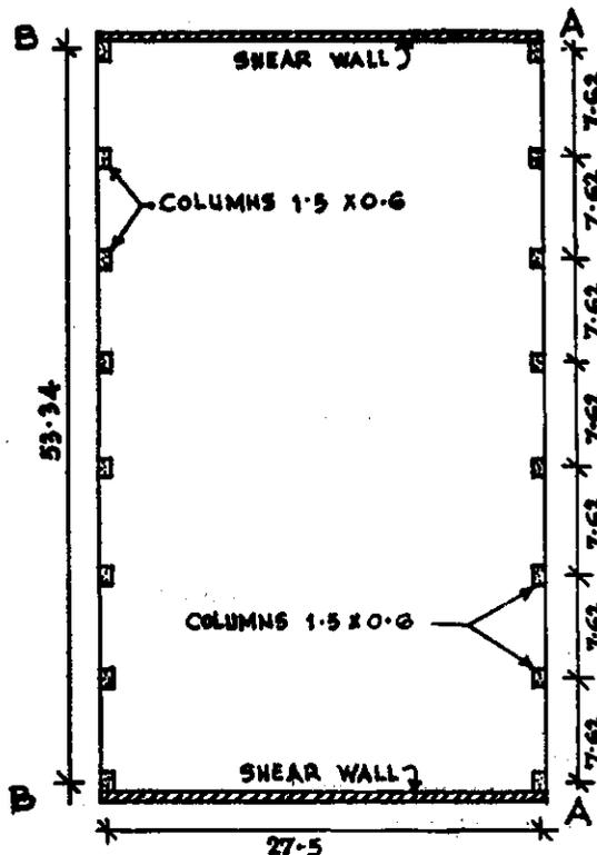
Fig. 1 Lay-out Plan
