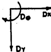
Fig. 3 Degrees of Freedom at a Typical Joint
