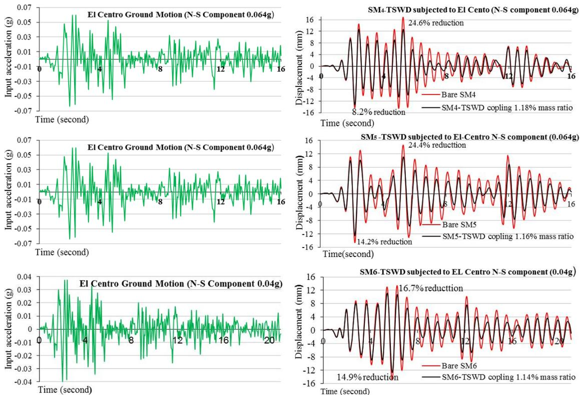
**Fig. 13 SM-TSWD coupling subjected to El Centro ground motion (N-S component)**
