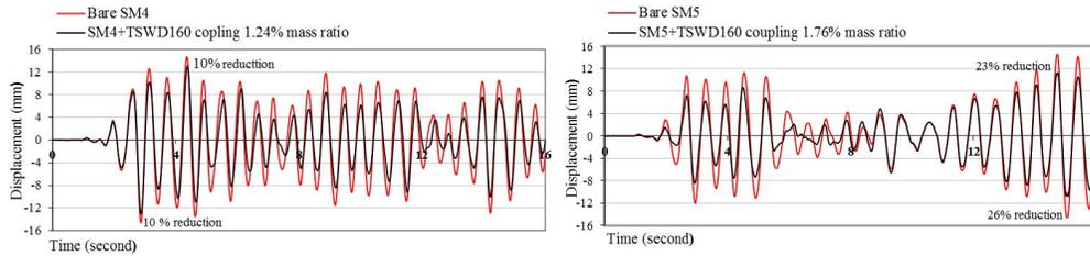
Fig. 16 SM<sub>4</sub>-TSWD<sub>275x280x160</sub> and SM<sub>5</sub>-TSWD<sub>350x350x160</sub> couplings subjected to BIS: 1893 compatible excitation
