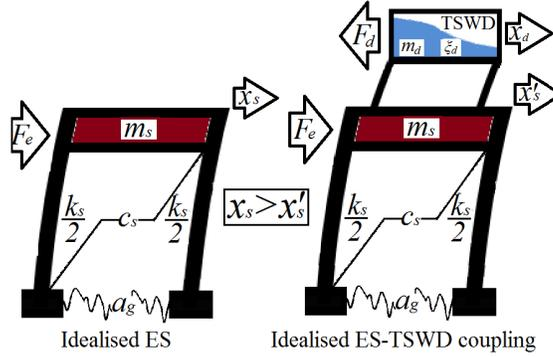
Fig. 6 Structure coupled with TSWD
