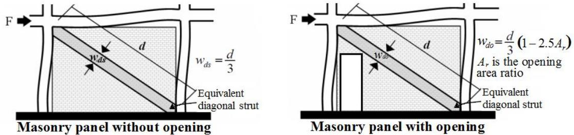
Fig. 2 Equivalent diagonal struts
