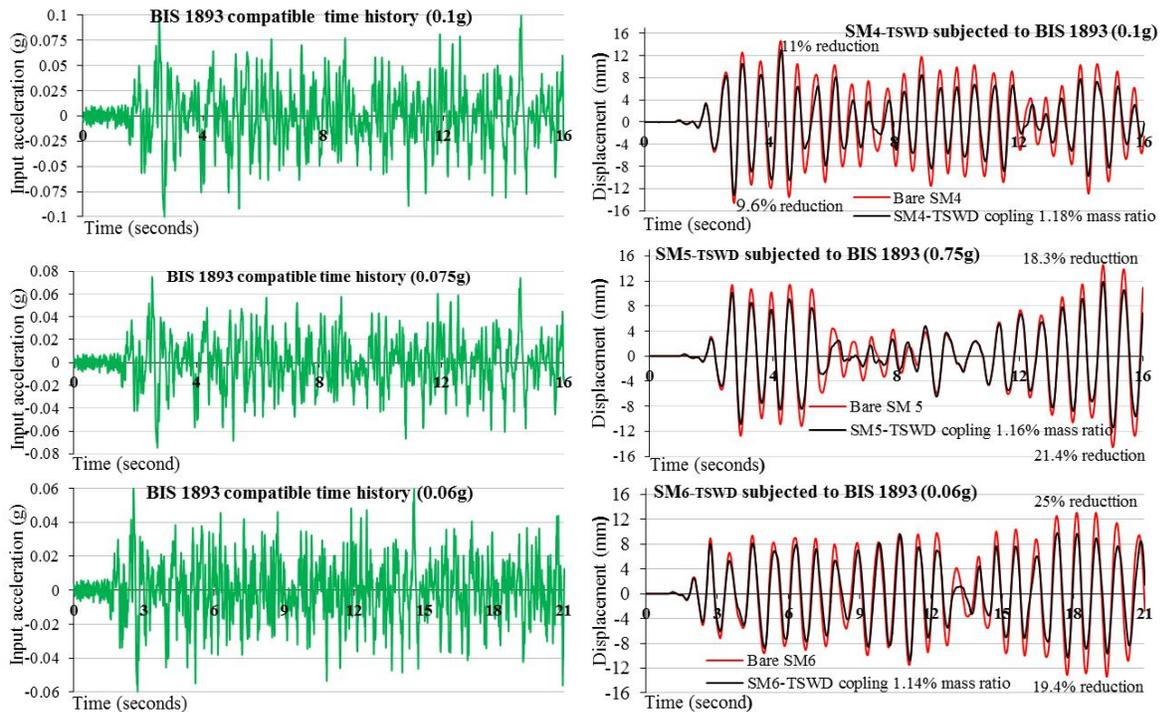
Fig. 15 SM-TSWD coupling subjected to BIS 1893 compatible time history
