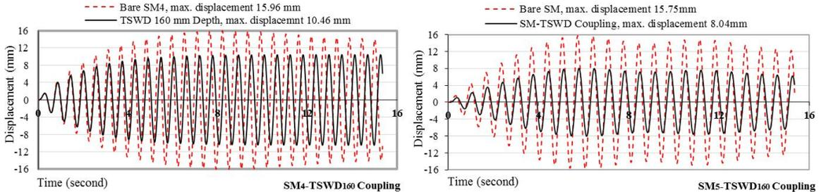
Fig. 12 SM<sub>4</sub>-TSWD<sub>275x280x160</sub> and SM<sub>5</sub>-TSWD<sub>350x350x160</sub> couplings subjected to harmonic excitation at base
