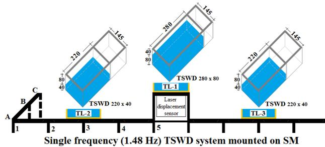
Fig. 17 Acrylic boxes converted as STSWD system
