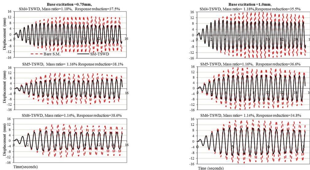
Fig. 10 SM<sub>4</sub>, SM<sub>5</sub>, SM<sub>6</sub> with optimal TSWDs subjected to resonant harmonic excitation
