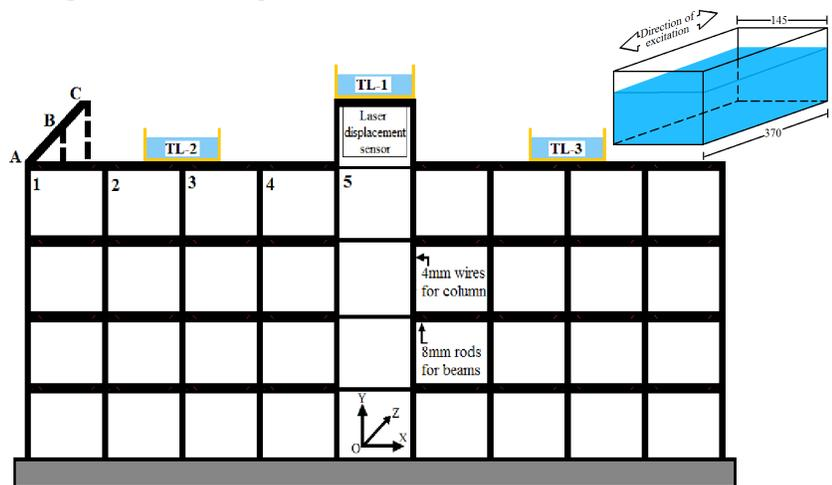
Fig. 8 Structural Skeleton of Scaled Model (SM)
