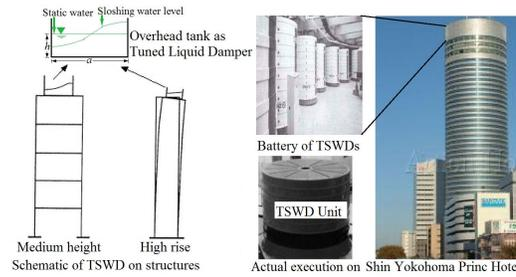
Fig. 1 TSWD on a structure
