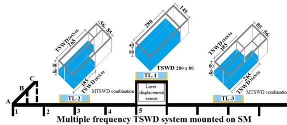
Fig. 18 Acrylic boxes converted as MTSWD System
