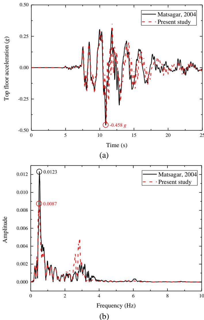
Fig. 6 Comparison of top floor acceleration obtained from the code and the published results for base-isolated structure in (a) time domain and (b) frequency domain
