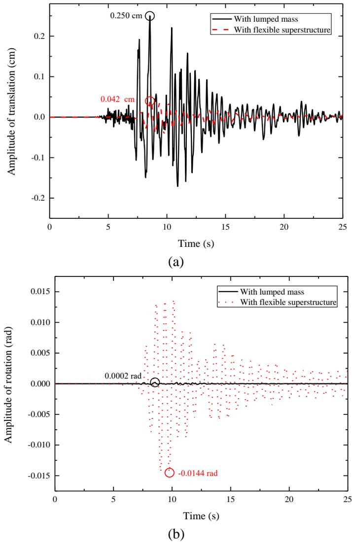
Fig. 9 Effect of flexibility on the soil (a) translation displacement, and (b) rotational displacement for a five-storey superstructure
