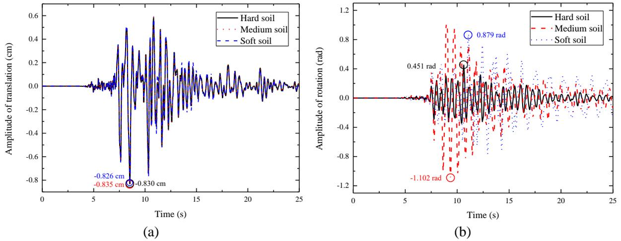
Fig. 11 Effect of soil types on the foundation response: (a) translation acceleration, and (b) rotation acceleration for a five-storey superstructure
