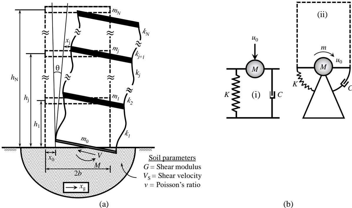
Fig. 1 (a) Mathematical model of  $N$ -storey structure (Wolf, 1997), (b) spring-dashpot-mass model of foundation for (i) translation and (ii) rotation
