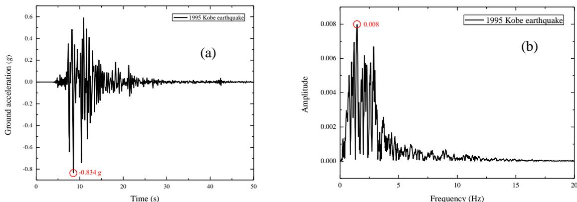
Fig. 7 The variation of the ground acceleration of the Kobe earthquake in (a) time domain and (b) frequency domain
