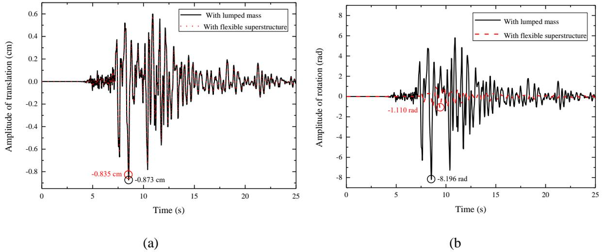
Fig. 8 Effect of flexibility on the soil (a) translation acceleration, and (b) rotation acceleration for a five-storey superstructure
