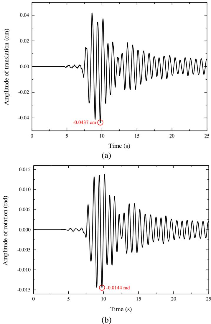
Fig. 3 Time variation of soil (a) translation displacement, and (b) rotation for a five-storey structure under Kobe, 1995 earthquake
