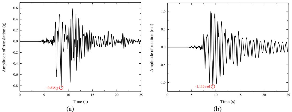
Fig. 2 Time variation of soil (a) translation acceleration, and (b) rotation acceleration for a five-storey structure under Kobe, 1995 earthquake
