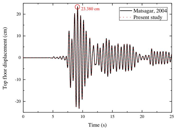
Fig. 5 Comparison of the time variation of top floor displacement obtained from the code and the published results
