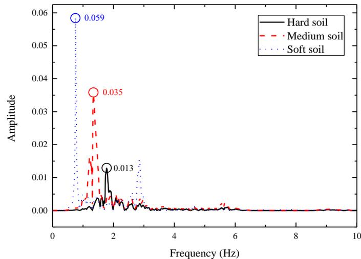
Fig. 13 Effect of soil types on the FFT response of foundation for a five-storey superstructure
