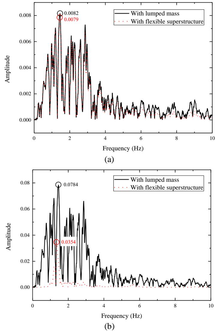
Fig. 10 Effect of flexibility on the FFT response of soil (a) translation acceleration, and (b) rotational acceleration for a five-storey superstructure
