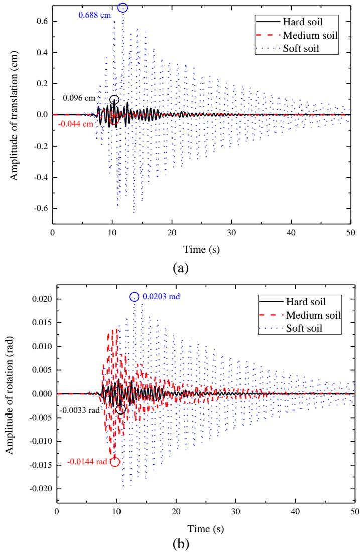
Fig. 12 Effect of soil types on the foundation response: (a) translation displacement, and (b) rotation displacement for a five-storey superstructure
