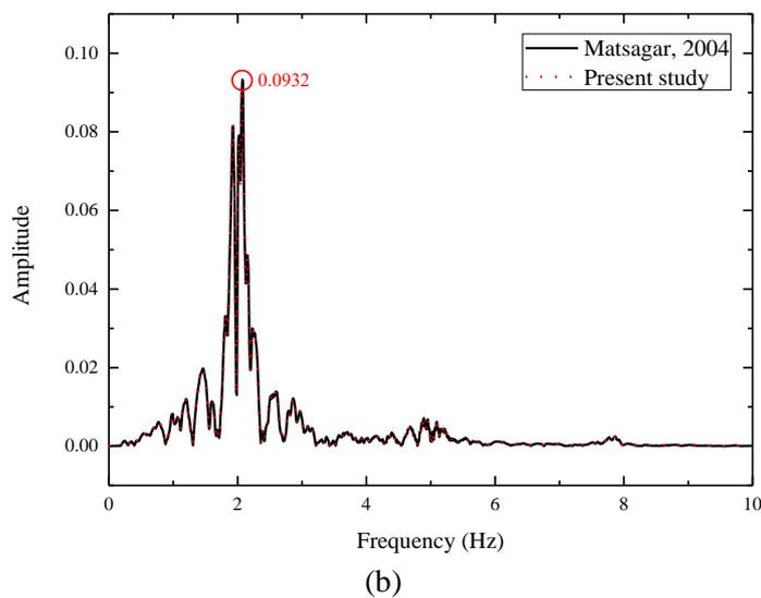
Fig. 4 Comparison of the top floor acceleration obtained from the code and the published results: (a) time domain and (b) frequency domain
