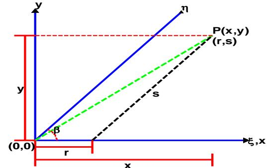
Fig.3 Point in global and local coordinate system
