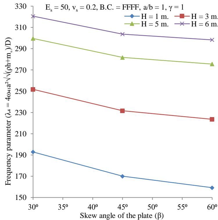
Fig. 10 Variation of frequency parameter of FFFF plate with the skew angle of the plate
