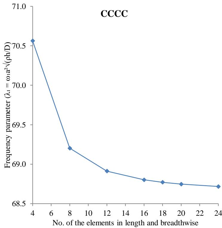
Fig. 5 First mode convergence study for a clamped plate's natural frequency
