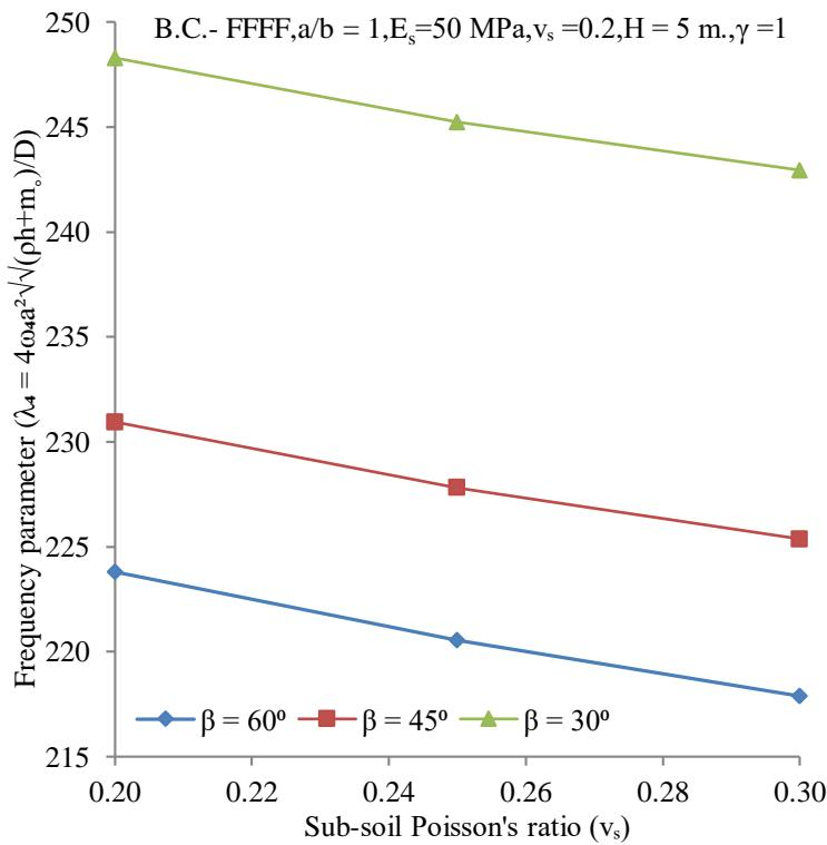
Fig. 16 Variation of frequency parameter of FFFF plate with sub-soil Poisson's ratio (v<sub>s</sub>)
