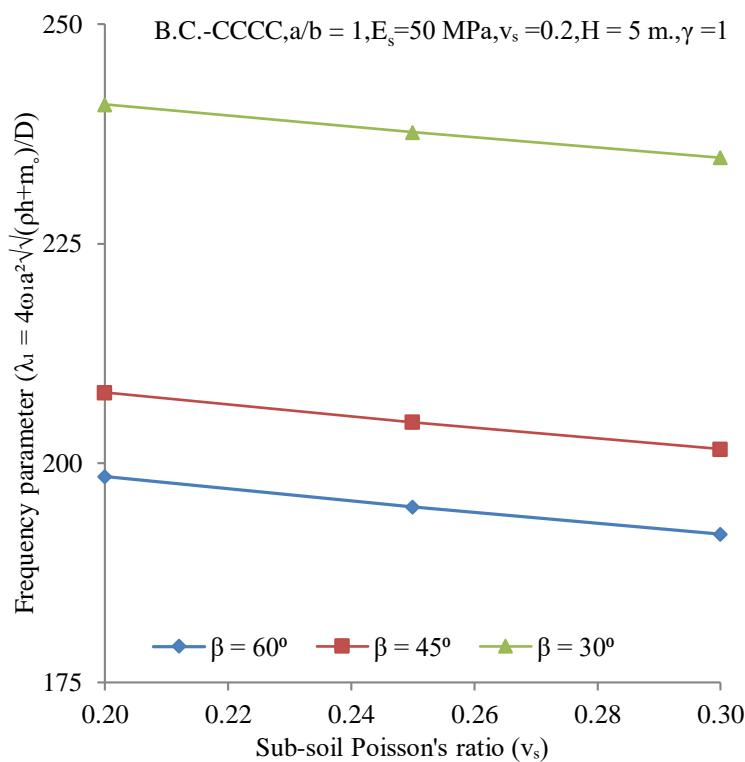
Fig. 14 Variation of frequency parameter of CCCC plate with the sub-soil Poisson's ratio ( $v_s$ )
