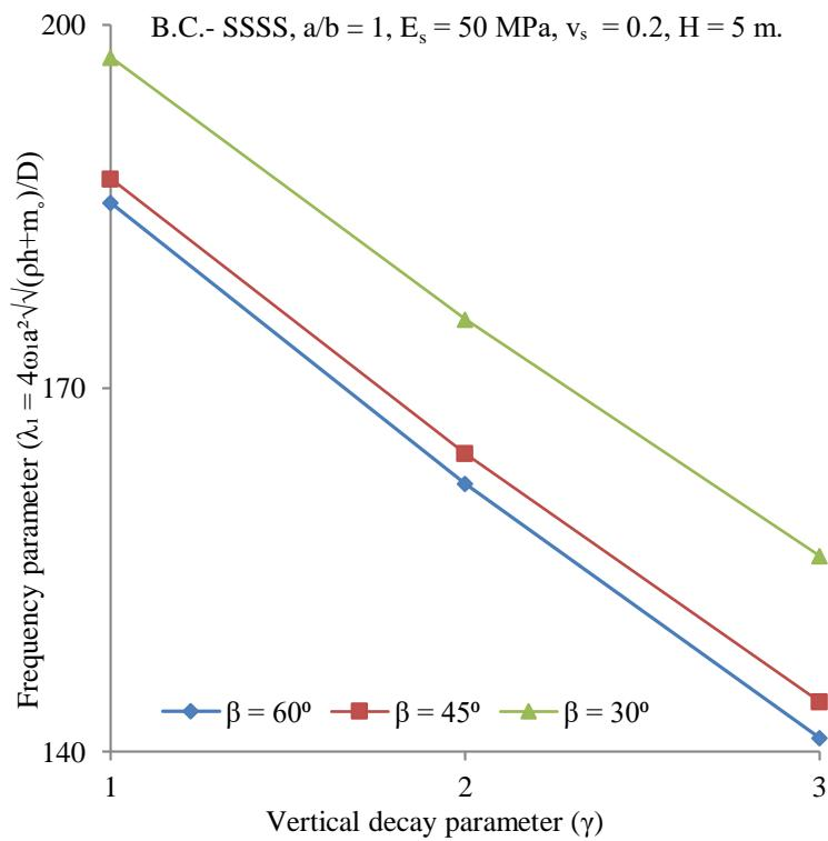
Fig. 12 Variation of frequency parameter of SSSS plate with the vertical decay parameter ( $\gamma$ )
