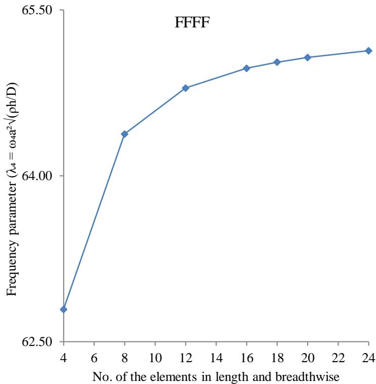
Fig. 7 Fourth mode convergence study for a free plate natural frequency
