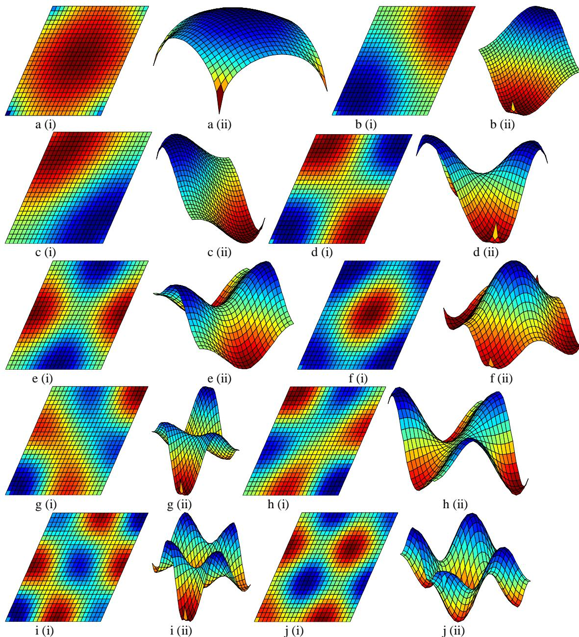
Fig. 17 First ten-mode shapes of the plate on elastic foundations for  $\gamma = 2$ ,  $H = 5$ ,  $\beta = 60^\circ$  and  $b/a = 1$
