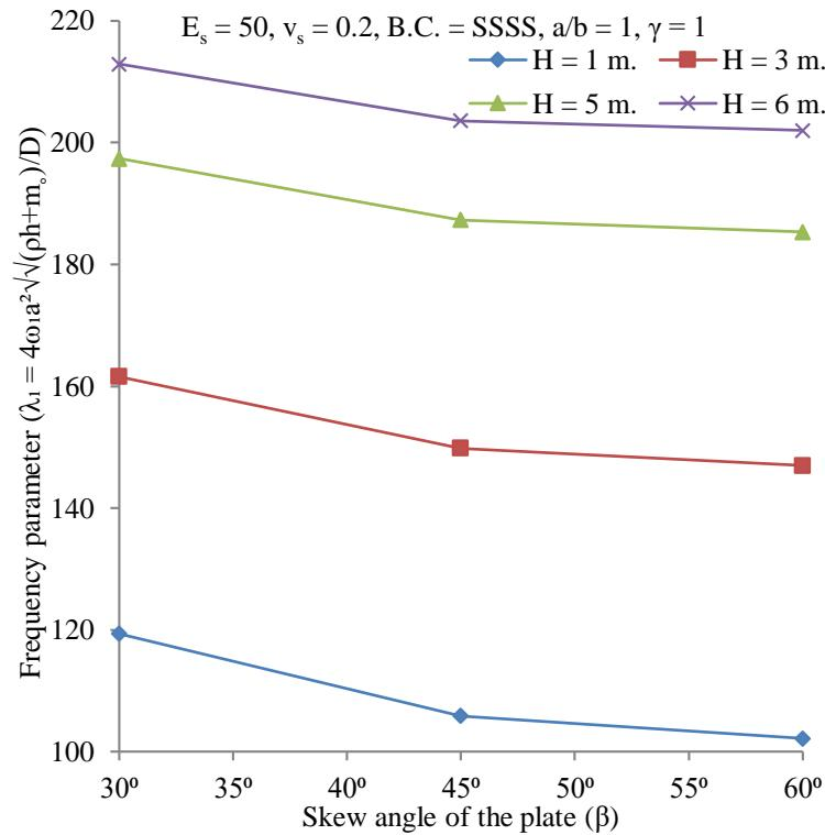
Fig. 9 Variation of frequency parameter of SSSS plate with the skew angle of the plate
