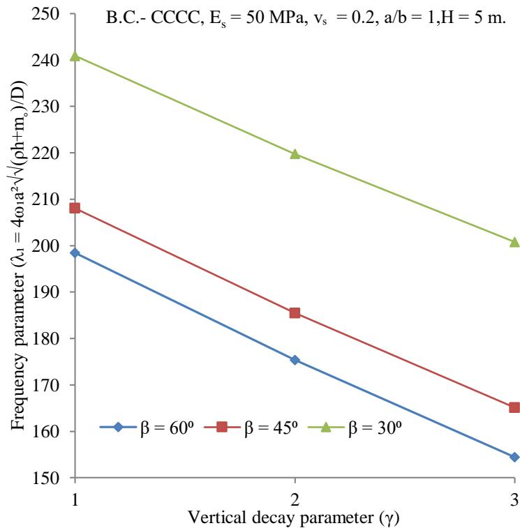
Fig. 11 Variation of frequency parameter of CCCC plate with the vertical decay parameter ( $\gamma$ )
