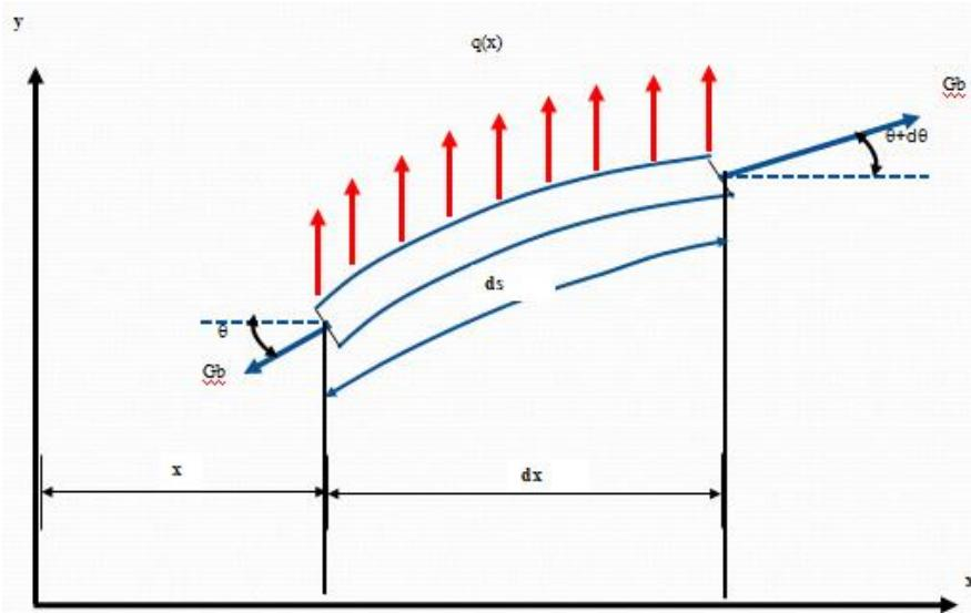
Fig. 4 Length of differential element 'dx' in deformed position, 'ds'
