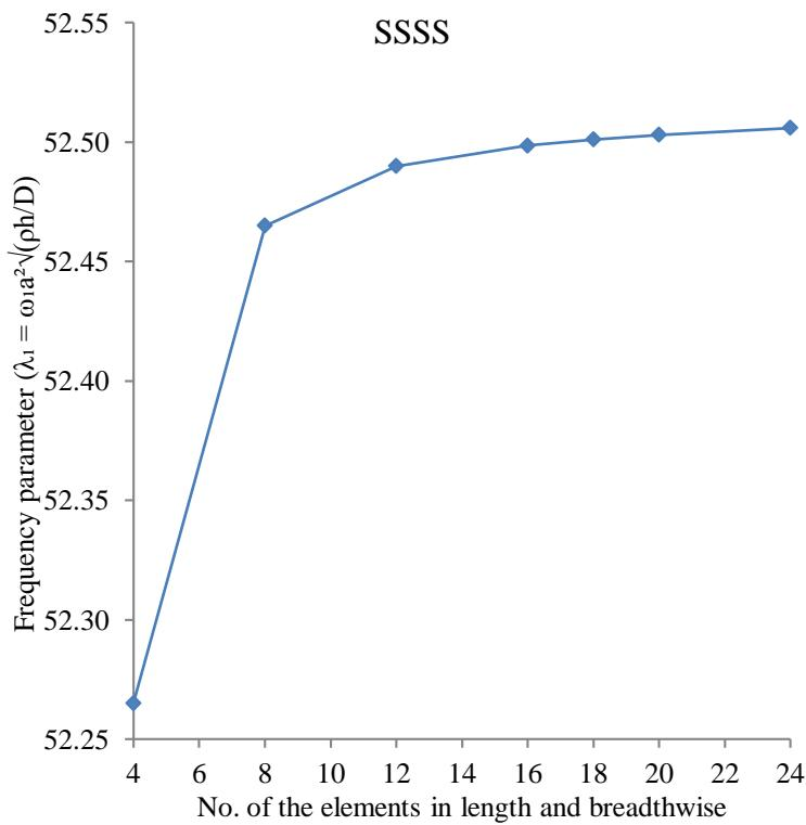
Fig. 6 First mode convergence study for a simply supported plate natural frequency
