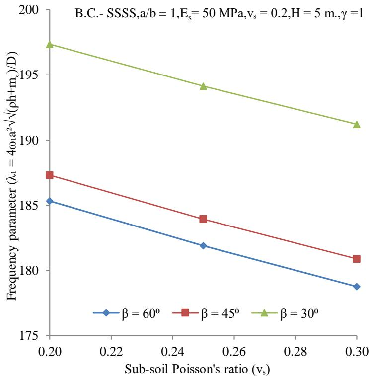
Fig. 15 Variation of frequency parameter of SSSS plate with the sub-soil Poisson's ratio (v<sub>s</sub>)
