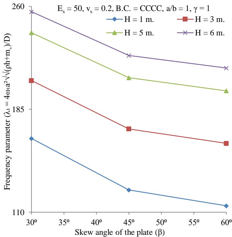
Fig. 8 Variation of frequency parameter of CCCC plate with the skew angle of the plate
