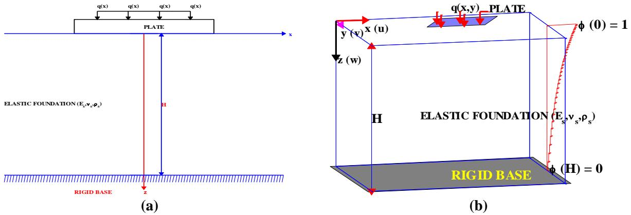
Fig. 1(a, b) Finite plates rest on a two-parameter Vlasov foundation
