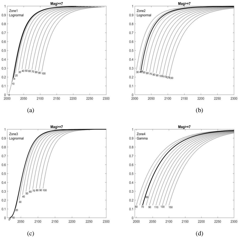
Fig. 3 Conditional probabilities for different elapsed time (t) for Earthquake  $M_w \geq 7.0$  (a) Zone 1, Lognormal (b) Zone 2, Lognormal (c) Zone 3, Lognormal (d) Zone 4, Gamma for different elapsed times ( $\tau$ ) indicated below the curves
