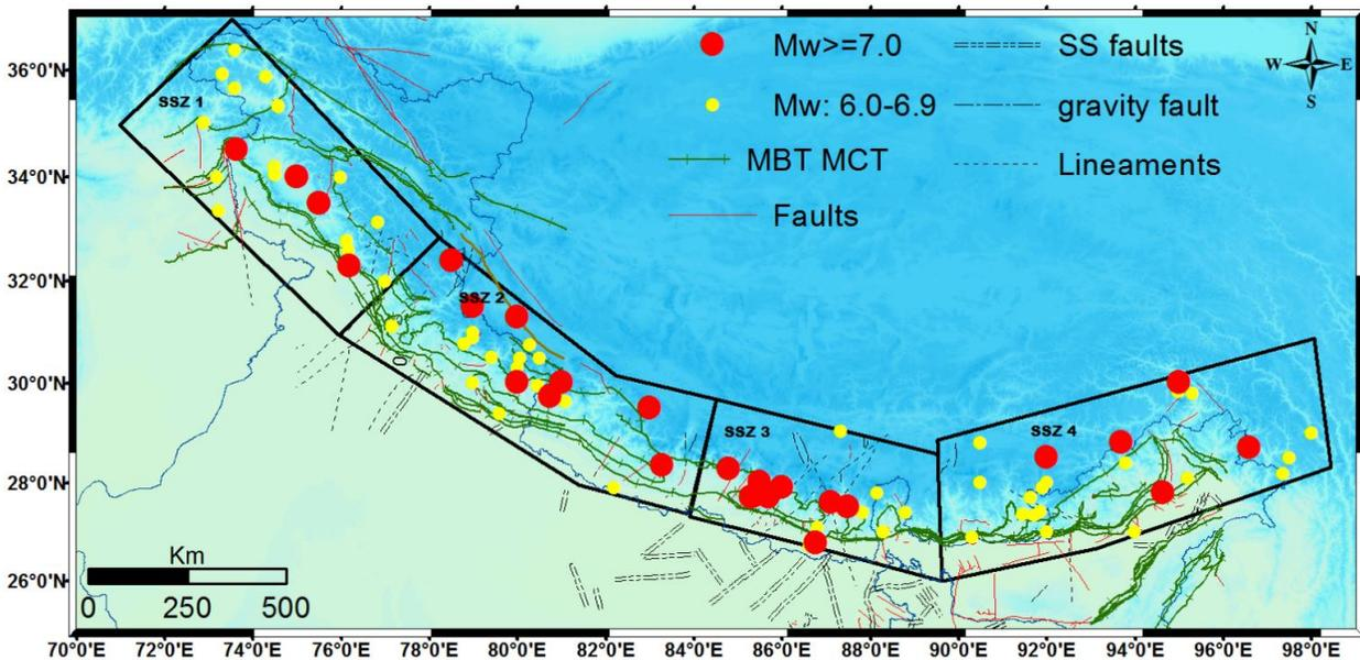
Fig. 1 Seismotectonics of the Himalayan seismic region showing major faults/folds/lineaments along with the locations of earthquakes of  $M_w \geq 6.0$ . This also shows the boundaries of four major SSZs for which probabilities of occurrences of future earthquakes have been calculated
