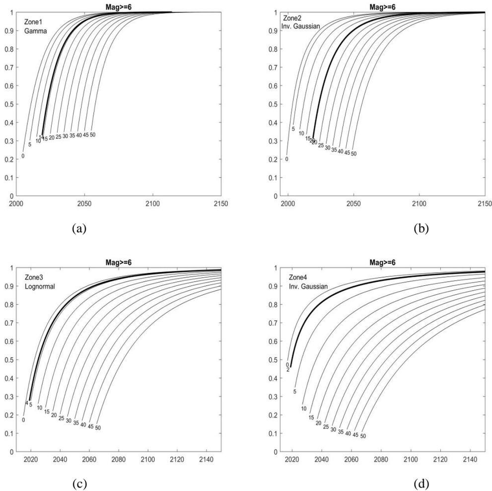
Fig. 2 Conditional probabilities for different elapsed time ( $t$ ) for Earthquake  $M \geq 6.0$  (a) Zone 1, Gamma (b) Zone 2, Inverse-Gaussian (c) Zone 3, Lognormal (d) Zone 4, Inverse-Gaussian for different elapsed times ( $\tau$ ) indicated below the curves
