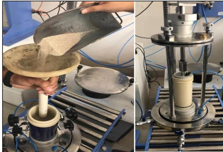
Fig. 3 Sample preparations using dry pluviation method
