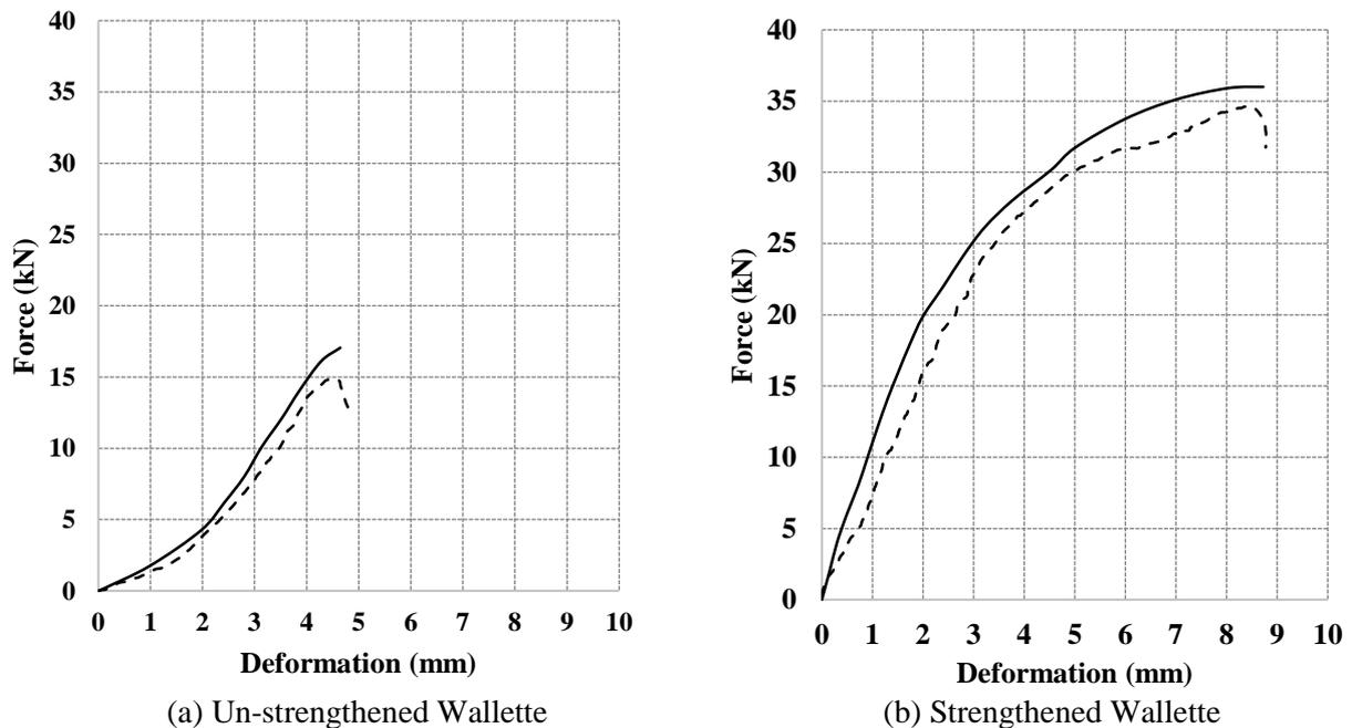
Fig. 4 Comparative force versus deformation diagram for the different pattern under out-of-plane loading (... Experimental, \_\_\_\_ Analytical)
