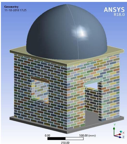
Un-Strengthened Masonry Model
