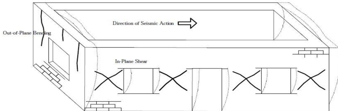
Fig. 1 Displacement of the building and typical collapse to structural walls [1]
