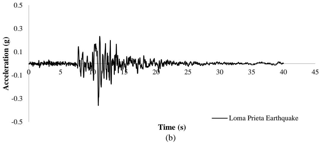
Fig. 5 Input ground acceleration (a) ISZ5, (b) Loma Prieta Earthquake
