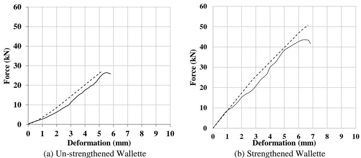
Fig. 2 Comparative force versus deformation diagram under pure in-plane loading (.... Analytical, \_\_ Experimental)
