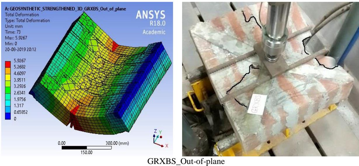
Fig. 3 Deformed shape of masonry wallette: numerical (left) with experimental (right) under in-plane and out-of-plane loading [11-12]
