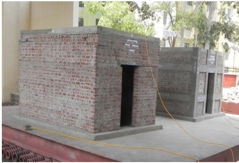
Fig. 3 Formation of cracks in traditional model whereas retrofitted model was intact after shock 2
