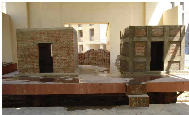
Fig. 2 Photograph showing the completed models on shock-table platform
