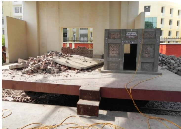
Fig. 4 Front view of the shock-table platform showing the traditional and retrofitted models after shock 3. The traditional model collapsed under this shock
