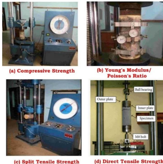
Fig. 19 Typical test setups for determining the (a) compressive strength; (b) Young's modulus and Poisson's ratio; (c) split tensile strength; and (d) direct tensile strength of dam concrete
