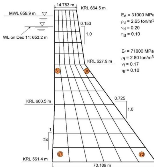
Fig. 10 FE idealization of the tallest non-overflow monolith of the Koyna dam used to compute the illustrative results by substructure method
