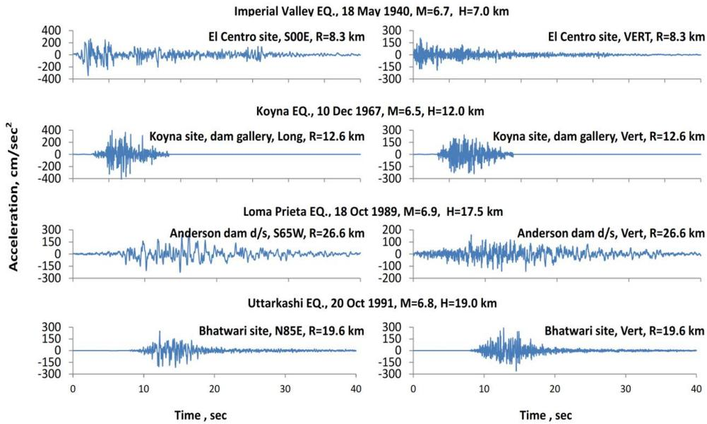
Fig. 16 Four sets of horizontal and vertical components of accelerograms used to compute the example results for illustrating the effects of stochastic nature of earthquake excitation
