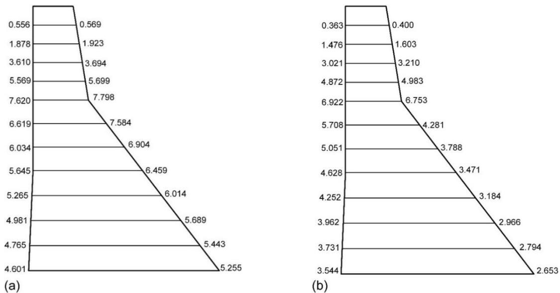
Fig. 3 Maximum principal stresses (in MPa) in the tallest monolith of Koyna dam with (a) static stresses excluded and (b) static stresses included
