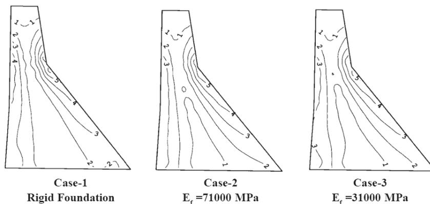
Fig. 12 Example results on the maximum principal stresses obtained by substructure method to illustrate the dam-foundation rock interaction effects
