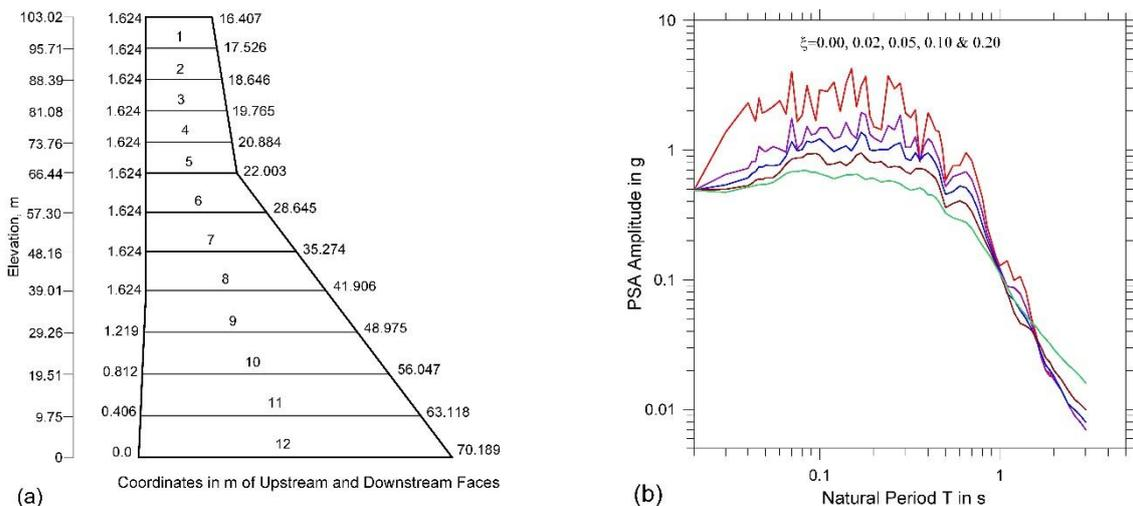
Fig. 2 (a) Tallest non-overflow monolith of Koyna dam divided into horizontal blocks for the purpose of response computation and (b) PSA spectra of the accelerogram used as input excitation
