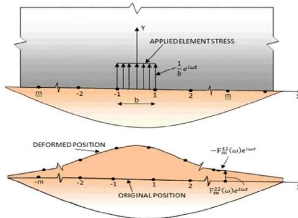
Fig. 9 Schematic illustration of the definition of flexibility influence (or compliance) coefficients  $F_m^{22}$  and  $F_m^{12}$  for vertically applied element load
