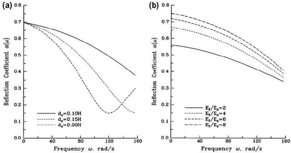
Fig. 8 Dependence of the wave reflection coefficient  $\alpha(\omega)$  on: (a) the thickness of the sedimentary layer at reservoir bottom; and (b) the modulus of elasticity of the rock below
