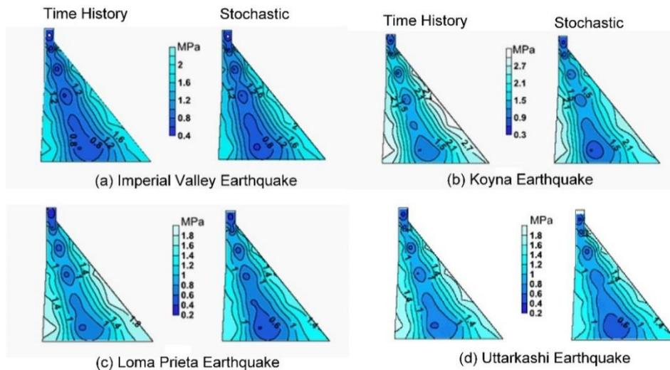
**Fig. 18 Comparison of the maximum principal stress contours based on statistical expected values of the highest peak with those based on the highest peak of the exact time history results with input excitations as the accelerograms of (a) Imperial Valley earthquake; (b) Koyna earthquake; (c) Loma Prieta earthquake; and (d) Uttarkashi earthquake**
