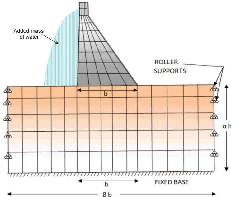
Fig. 4 Standard FE analysis by including a limited portion of the foundation with no mass and fixed base, and the hydrodynamic forces modeled by a mass of water attached to the upstream face of the dam
