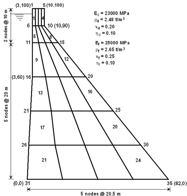
Fig. 15 FE idealization of the typical dam section used to compute the example results for illustrating the effects of stochastic nature of earthquake excitation
