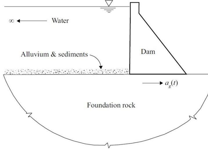
Fig. 6 Dam-foundation-reservoir system in substructure modeling (after [9])
