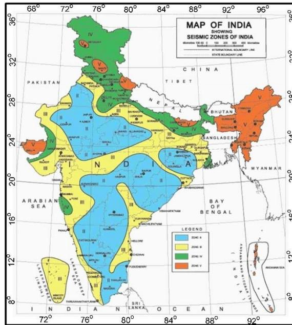
Fig. 1 Seismic zoning map of India as per IS: 1893 (Part 1)-2016 [16]
