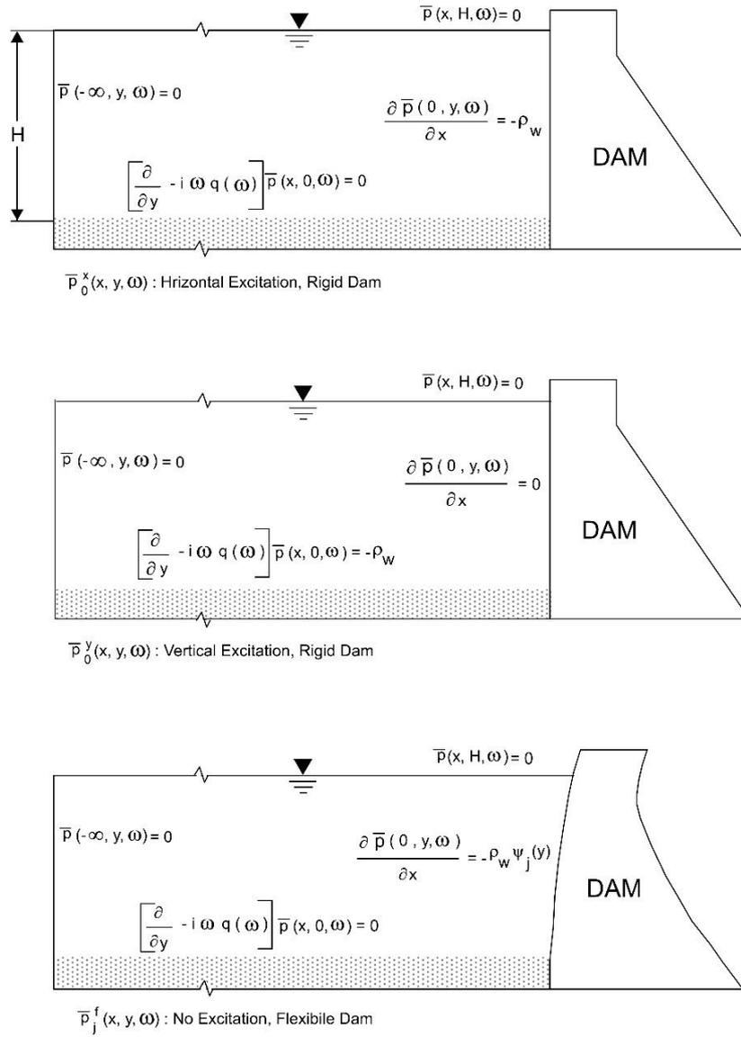
Fig. 7 Illustration of the boundary conditions used for the estimation of three different contributions to the hydrodynamic forces
