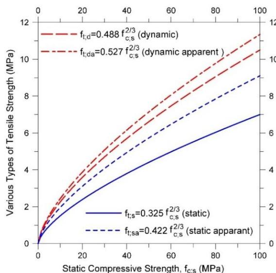
Fig. 20 Various types of tensile strength of dam concrete as a function of the static compressive strength (modified after Raphael [56])
