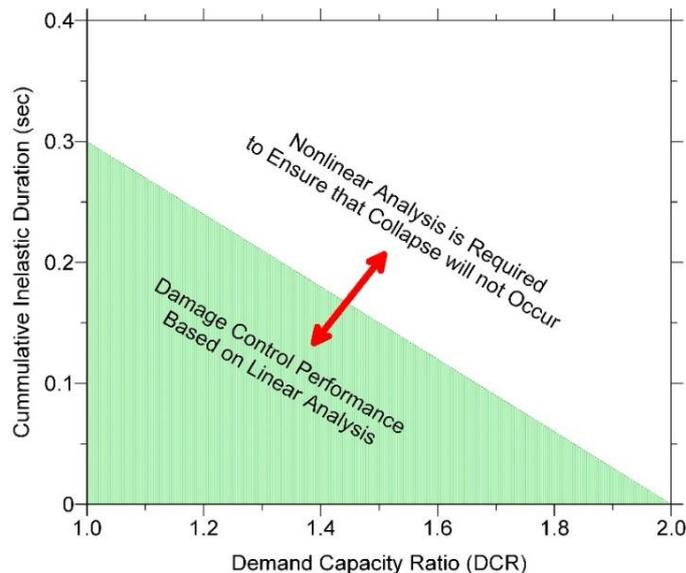
Fig. 21 Performance curve for concrete gravity dams analyzed by linear elastic time-history method (after [6])
