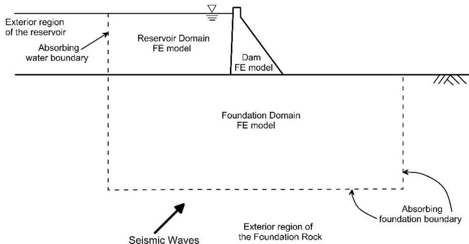
Fig. 5 Dam-reservoir-foundation system with truncated foundation and reservoir domains with wave-absorbing boundaries
