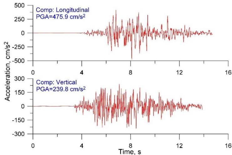
Fig. 11 Longitudinal and vertical components of the accelerograms recorded at the foundation gallery of the Koyna dam from the earthquake of 11 December 1967 with magnitude 6.5
