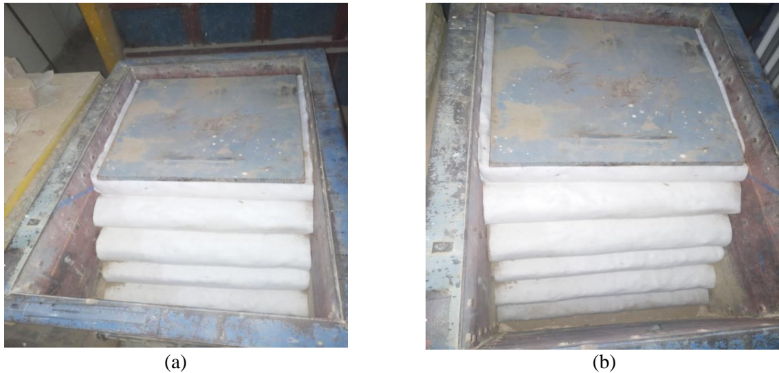
Fig. 5 Finished wrap-faced wall profiles: (a) five-layer configuration; (b) six-layer configuration
