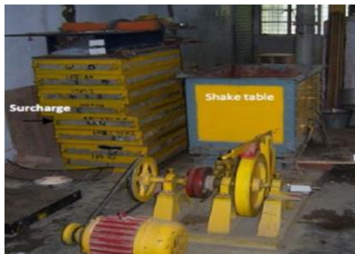
Fig. 2 View of shake table and surcharge weights
