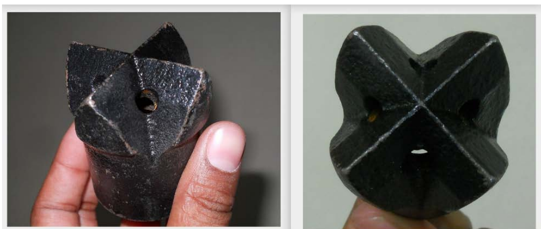
Fig. 9 (b) Closed view of cutting bit of Self drilling anchor
