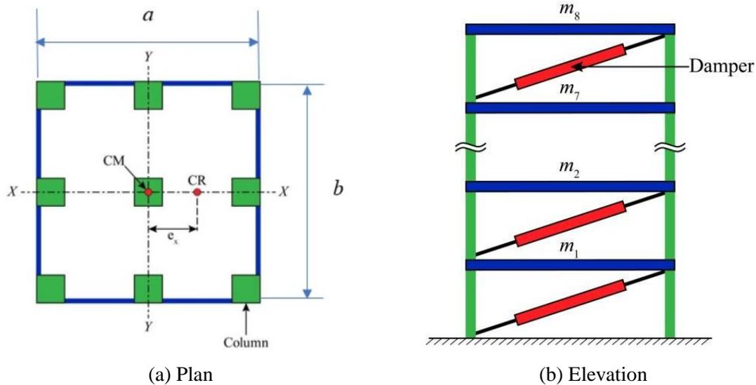
Fig. 1 Schematic plan and elevation of asymmetric-plan building
