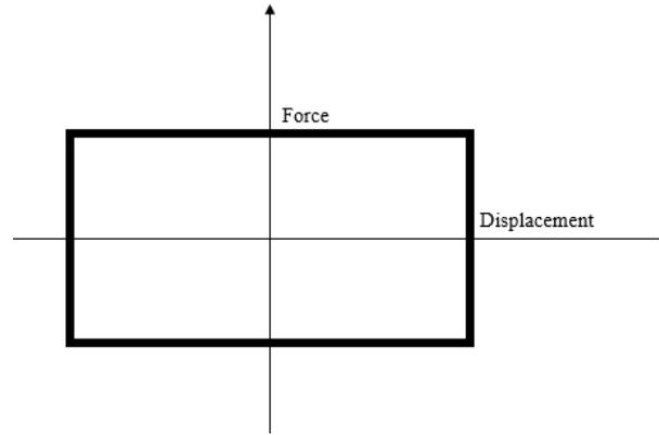
Fig. 4 Force-displacement loop for friction damper
