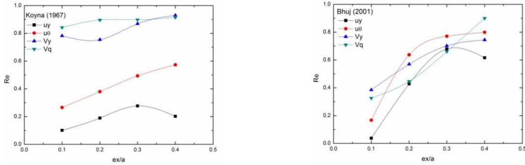
Fig. 6 Variation of response ratio ( $R_e$ ) with eccentricity ratio ( $e_x/a$ ) for Koyna and Bhuj earthquakes
