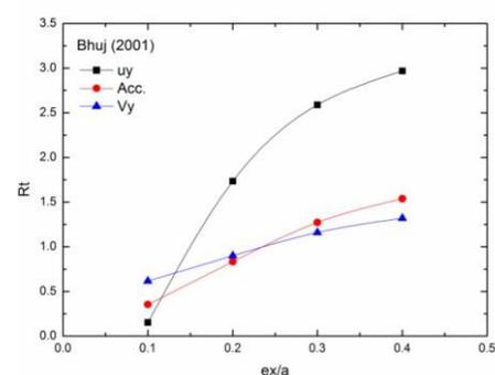
Fig. 8 Variation of response ratio ( $R_t$ ) with eccentricity ratio ( $e_x/a$ )
