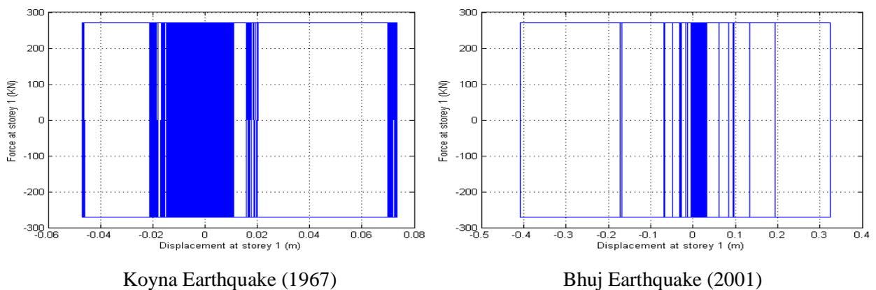
**Fig. 5 Force displacement loops for Koyna (1967) and Bhuj (2001) earthquakes**
