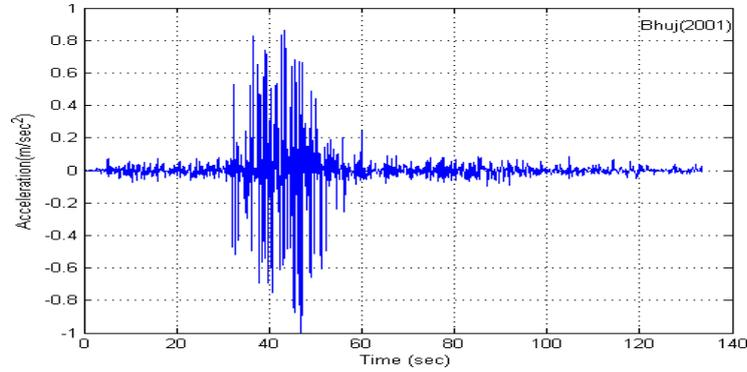
Fig. 3 Acceleration time history for Bhuj earthquake (2001)
