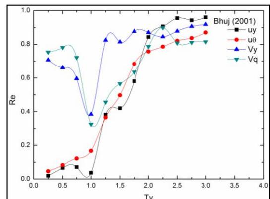
Fig.7 Variation of response ratio ( $R_e$ ) with time period ( $T_y$ )
