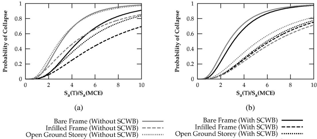
Fig. 10 Fragility curves for RC frame buildings considered in the present study (a) 4-storey, and (b) 8-storey
