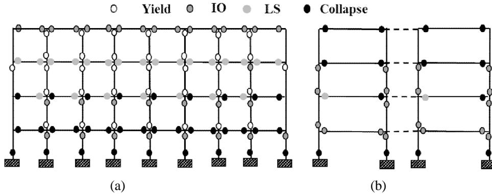
Fig. 7 Collapse mechanism of 4-storey RC bare frame building designed as SMRF with consideration of SCWB ratio, as per relevant Indian Standards: (a) typical longitudinal frame, and (b) typical transverse frame
