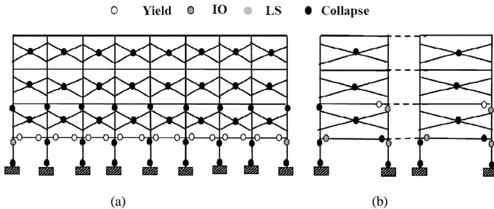
Fig. 9 Collapse mechanism of 4-storey open ground storey building designed as SMRF with consideration of SCWB ratio, as per relevant Indian Standards: (a) typical longitudinal frame, and (b) typical transverse frame
