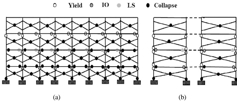
Fig. 8 Collapse mechanism of 4-storey uniformly infilled RC frame building designed as SMRF with consideration of SCWB ratio, as per relevant Indian Standards: (a) typical longitudinal frame, and (b) typical transverse frame
