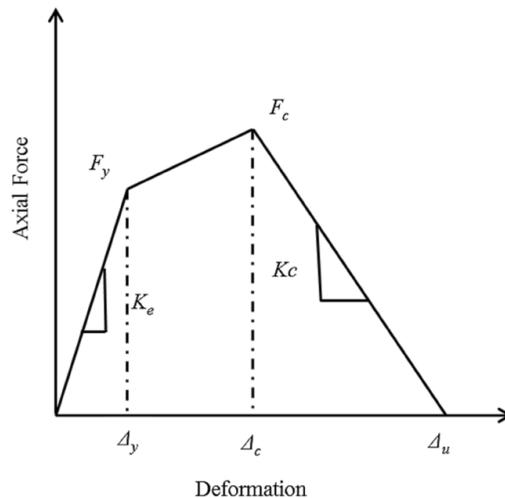
Fig. 3 Generalized force-deformation behavior of infill strut (Burton and Deierlein 2014)
