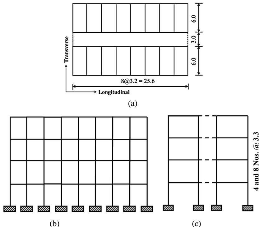
Fig. 1 (a) Generic plan, (b) front, and (c) side elevation of the considered buildings (The dotted lines represent the floor slabs boundaries, which are assumed to be rigid in its plane). All dimensions are in meter.
