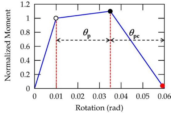
Fig. 2 Generalized force-deformation behaviour for RC frame elements
