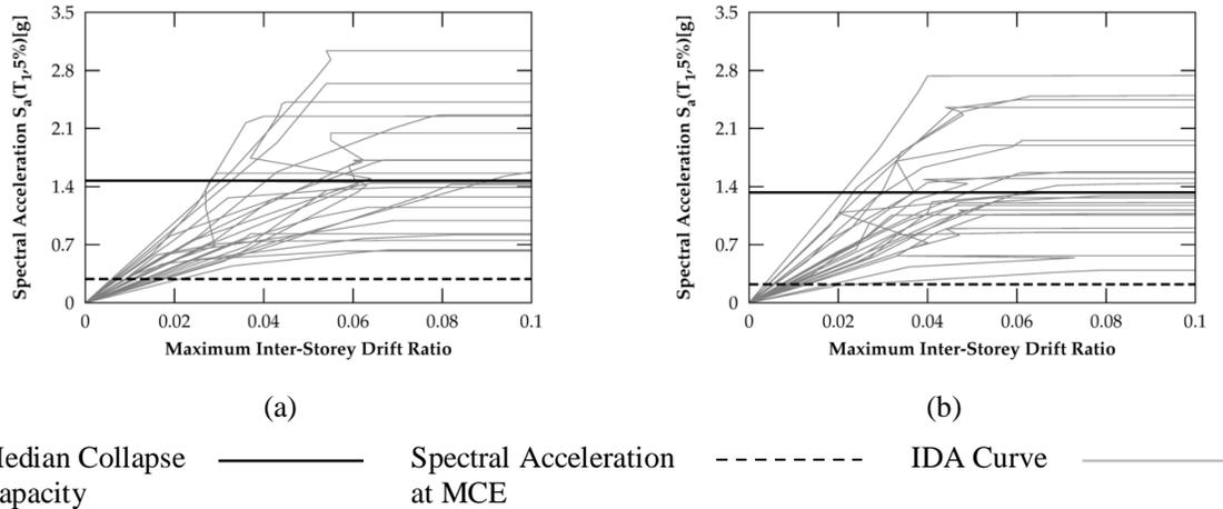
Fig. 6 Dynamic capacity curves (for a suite of 22 far-field ground-motion records) of open ground storey buildings designed as SMRF with consideration of SCWB ratio, as per relevant Indian Standards, for: (a) 4-storey, and (b) 8-storey
