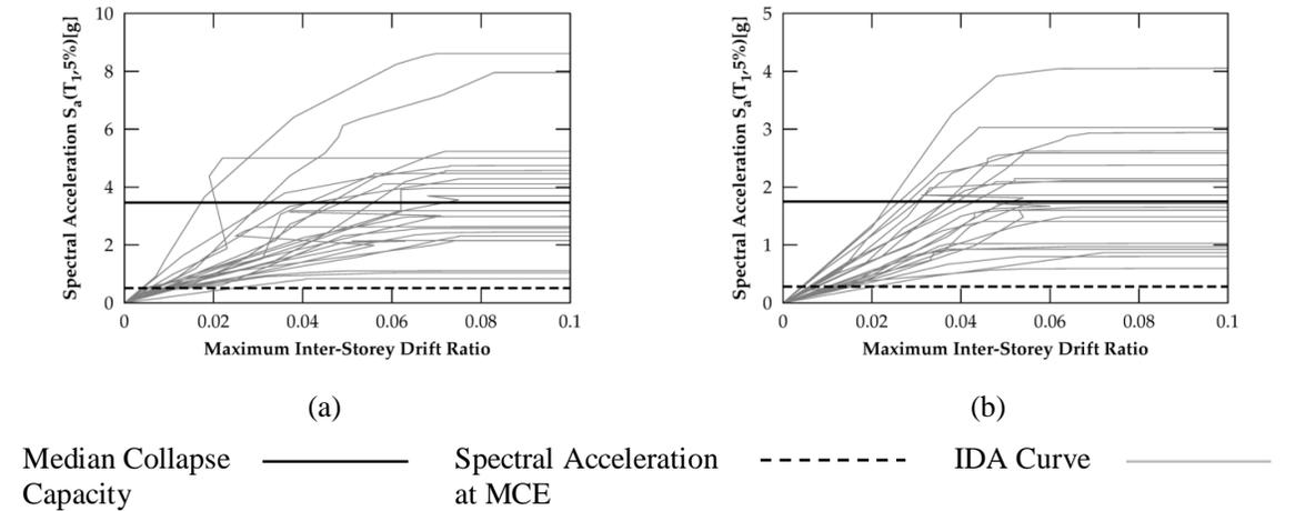
Fig. 5 Dynamic capacity curves (for a suite of 22 far-field ground-motion records) of uniformly infilled RC frame buildings designed as SMRF with consideration of SCWB ratio, as per relevant Indian Standards, for: (a) 4-storey, and (b) 8-storey
