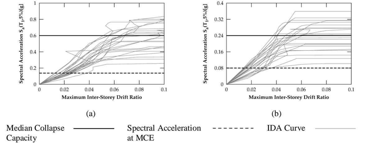
Fig. 4 Dynamic capacity curves (for a suite of 22 far-field ground-motion records) of RC bare frame buildings designed as SMRF with consideration of SCWB ratio, as per relevant Indian Standards, for: (a) 4-storey, and (b) 8-storey
