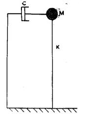
Fig. 3. Equivalent Dynamic of a Single Storey, Single Bay Infilled Frame.
