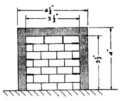
Fig. 2. Infilled Frame with Shear Connectors.
