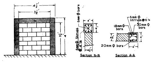
Fig. 1a. Infilled Frame without Shear Connectors.
