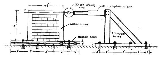
Fig. 5a. Testing Arrangement for Loading Infilled Frames Laterally
