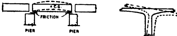
Fig. 1. Vertical accelerations due to bending of piers in longitudinal direction
