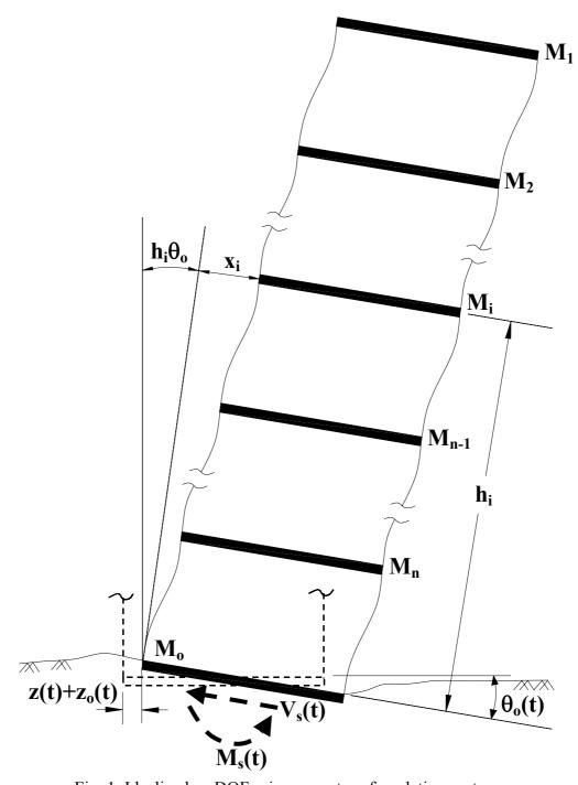
Fig. 1 Idealized *n* -DOF primary system-foundation system
