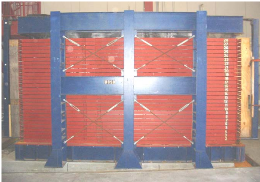
Fig. 4 The UCSD medium size laminar box (Jakrapiyanun, 2002)
