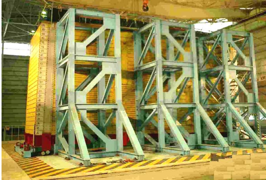
Fig. 3 The NIED large size laminar box (Tokimatsu and Suzuki, 2004)
