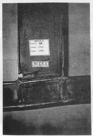
Fig. 14 Failure mode of a fully welded connection (BCC5)
