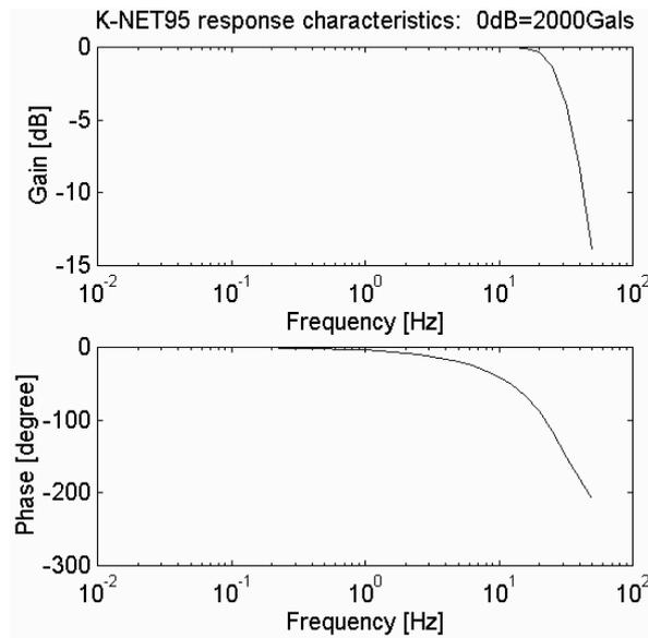
Fig. 2 Response characteristic curves of K-NET95 accelerographs<sup>1</sup>
