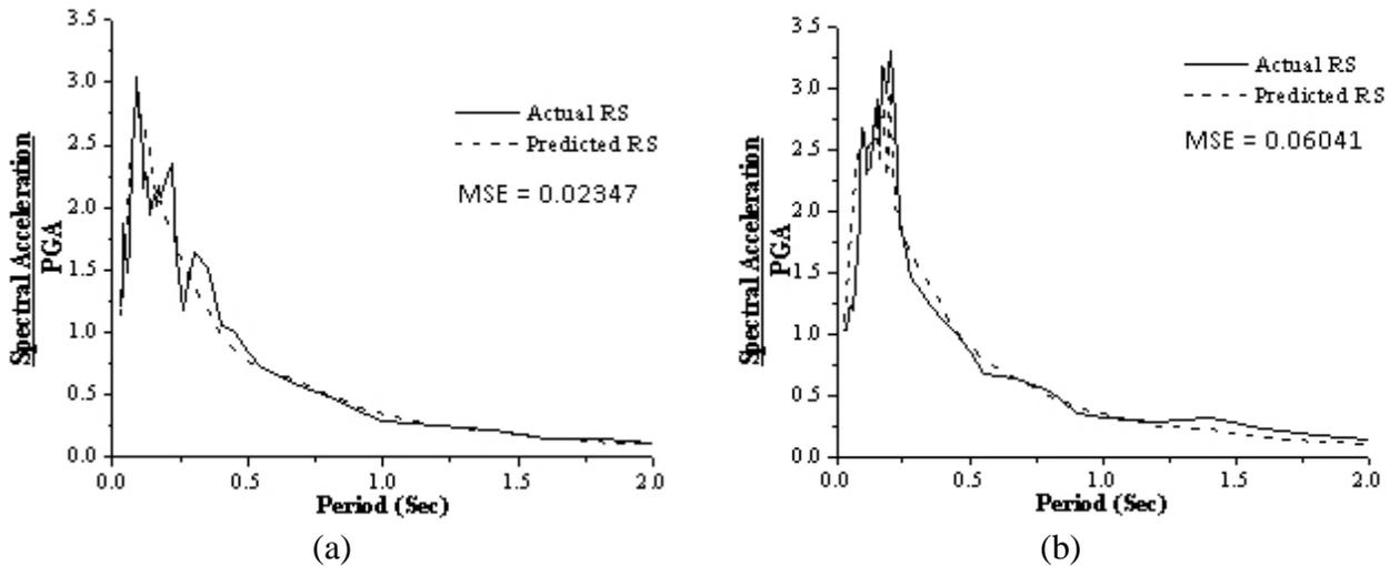
Fig. 8 Typical plots of acceleration response spectra predicted by ANN with three inputs for (a)  $M = 5.2, H = 42 \text{ km}, \bar{v}_s = 455.5 \text{ m/s}$  and (b)  $M = 5.1, H = 39.6 \text{ km}, \bar{v}_s = 345.8 \text{ m/s}$
