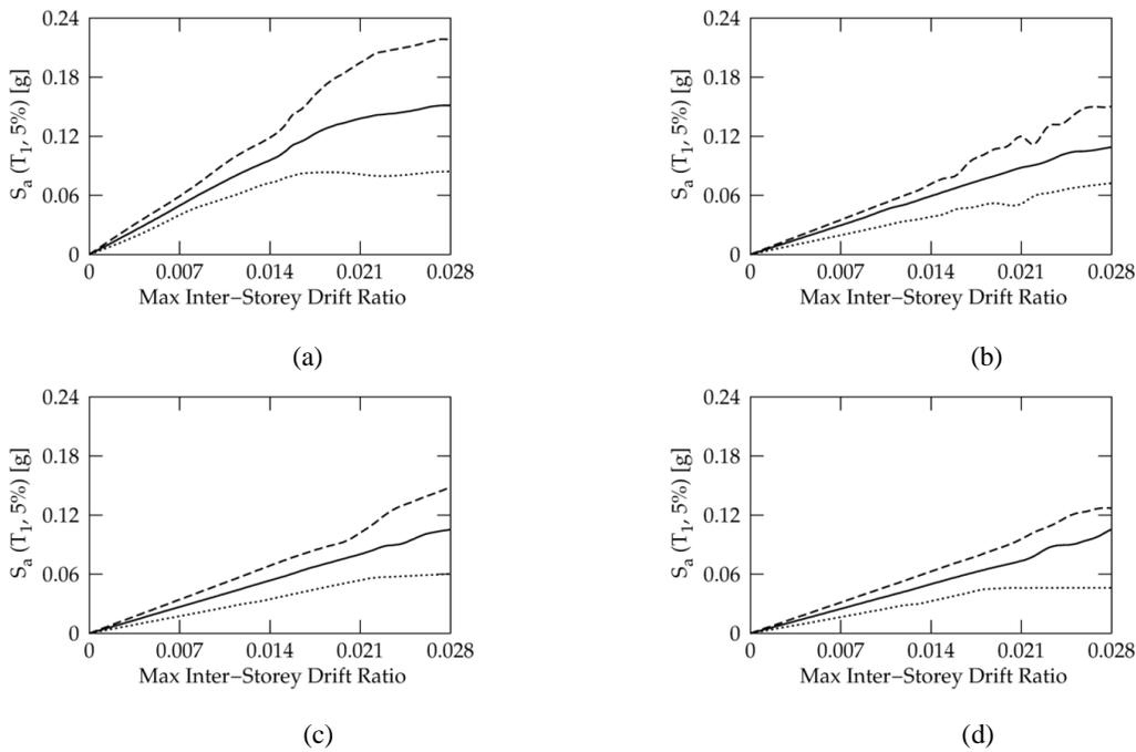
Fig. 4 Dynamic capacity curves for 8-storey buildings: (a) Regular symmetric building, (b) 5% Mass-eccentric building, (c) 10% Mass-eccentric building, and (d) 15% Mass-eccentric building
