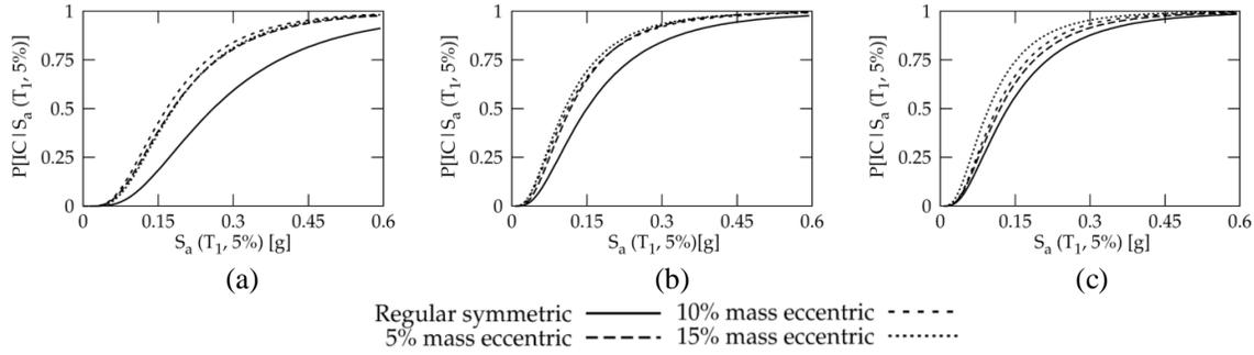
Fig. 6 Fragility curves for regular symmetric and mass-eccentric buildings: (a) 4-storey buildings, (b) 8-storey buildings, and (c) 12-storey buildings.  $P[IC | S_a(T_1, 5\%)]$  represents the probability of incipient collapse for a given spectral acceleration demand,  $S_a(T_1, 5\%)$
