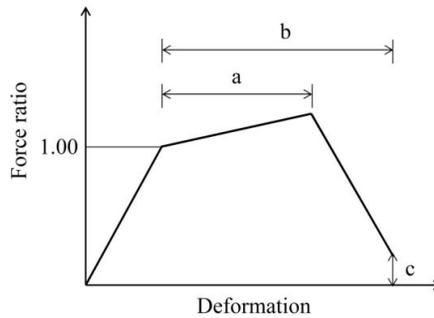
Fig. 2 Force-deformation curve for members under flexure. (Values of modelling parameters a, b, and c are provided in Table 3)
