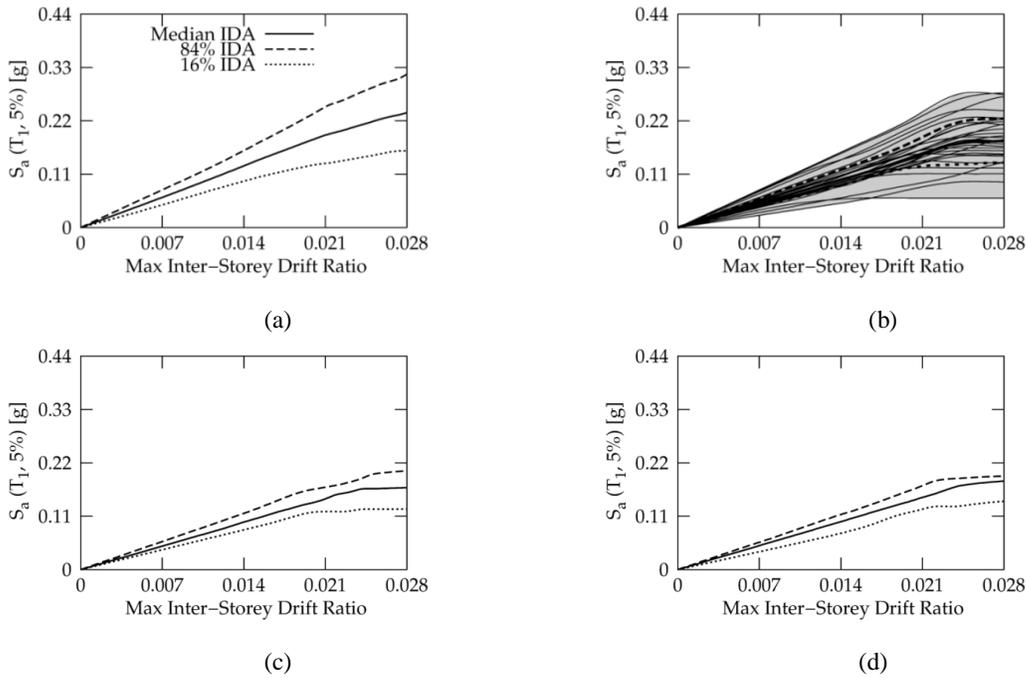
Fig. 3 Dynamic capacity curves for 4-storey buildings: (a) Regular symmetric building, (b) 5% Mass-eccentric building, (c) 10% Mass-eccentric building, and (d) 15% Mass-eccentric building
