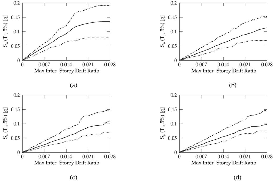
Fig. 5 Dynamic capacity curves for 12-storey buildings: (a) Regular symmetric building, (b) 5% Mass-eccentric building, (c) 10% Mass-eccentric building, and (d) 15% Mass-eccentric building
