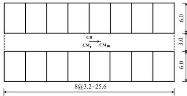
Fig. 1 Plan of the considered building models (CR - centre of rigidity, CM<sub>r</sub>- centre of mass of regular building, and CM<sub>m</sub> - centre of mass of mass-eccentric building, longer and shorter dimensions are considered along x and y directions, respectively).
