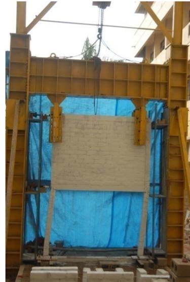
Fig. 21 Frame at failure stage indicating rigid body displacement of upper storey- MI-RC frame model with open ground storey
