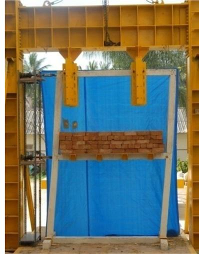
Fig. 19 Frame at failure stage. - Bare RC frame model
