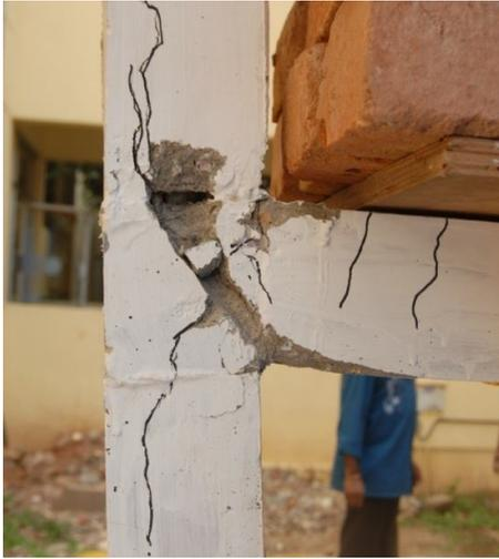
Fig. 18 Formation of plastic hinge at bottom storey beam-column junction - Bare RC frame model
