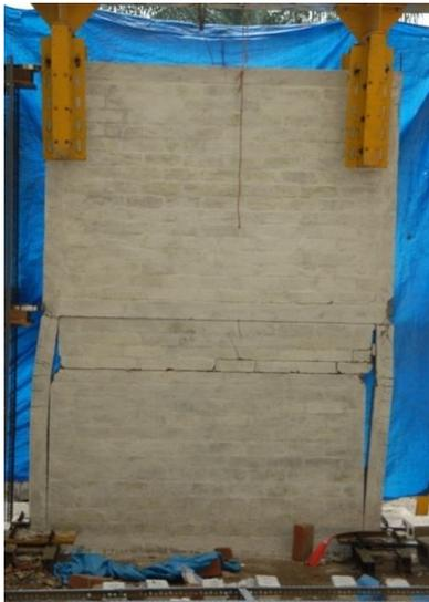
Fig. 20 Sliding shear of masonry leading to shear failure of column – MI-RC frame model
